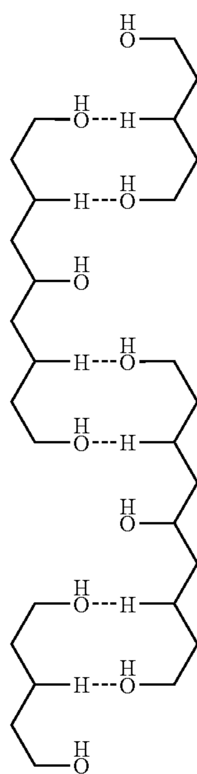
The gaps created in the linked polymer chain allow molecules of polar solvents (such as water molecules in soapy water) to interrupt the hydrogen bonds and solvate the cured modified RMA flux residue within the gaps of the long misaligned chain, similar to the non-polar/hydrocarbon solvents used to solvate hydrogen bonds as previously discussed. The resulting soapy organic slurry can be removed by mechanical blotting with a cloth or by a water rinse.
