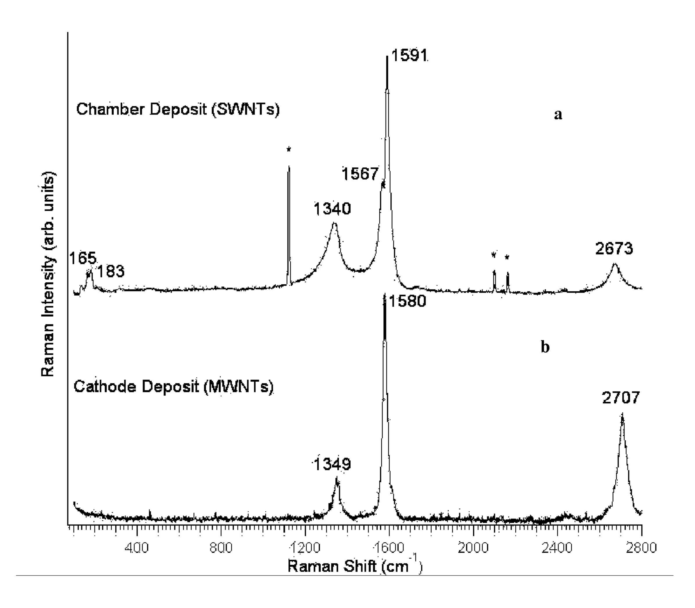
**Fig.5** Room temperature Raman spectra of the chamber and cathode deposit. Chamber deposit (a) shows the presence of SWNTs and The Cathode deposit(b) shows the presence of MWNTs
