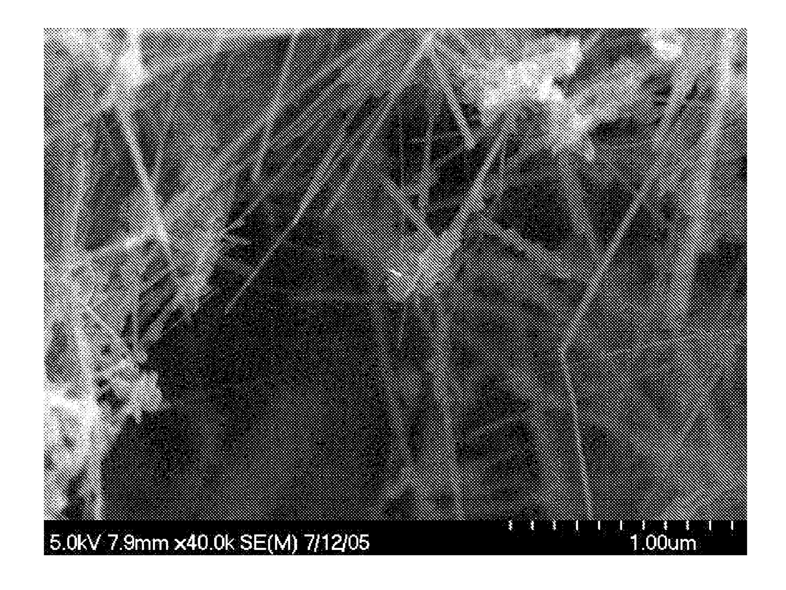
Fig.4 SEM micrograph of the cathode deposit showing the presence of straight MWNTs
