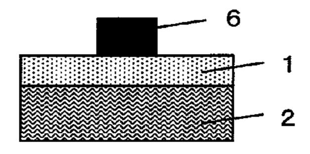
(e) Laminating and curing a resin film for forming an upper cladding layer
