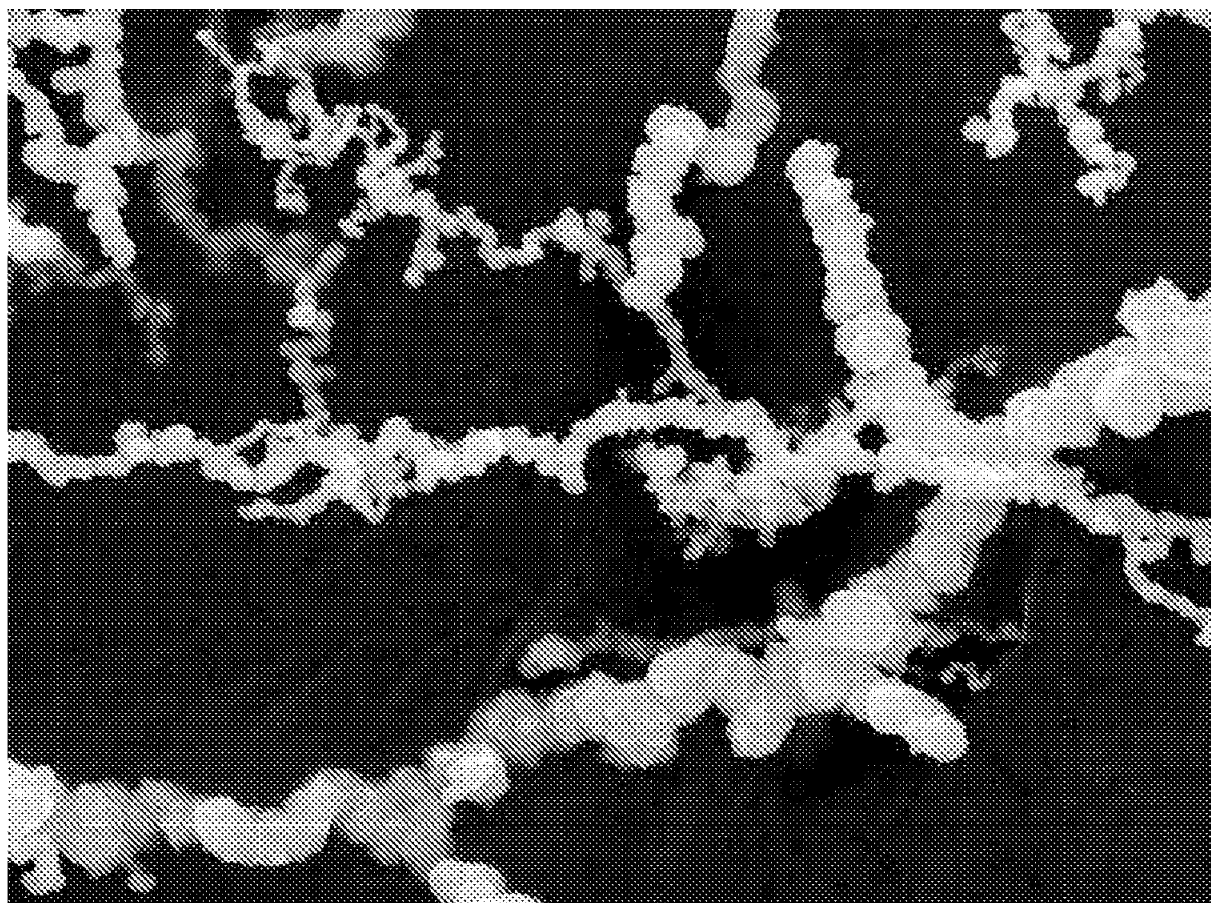
Nickel 500-nanometer branching nanostrands of FIG. 2, enlarged 10,000 times
