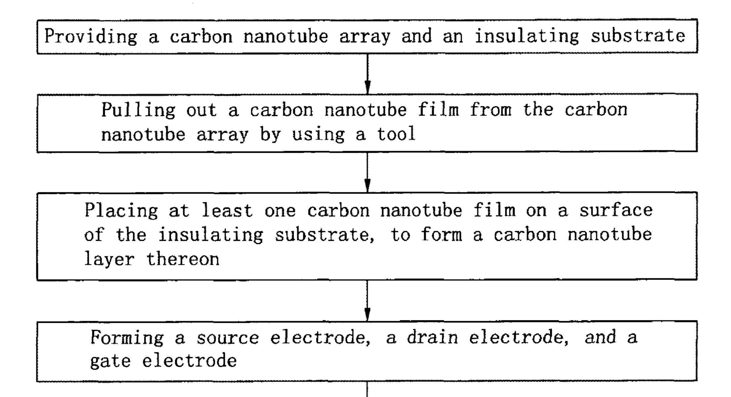
Covering the carbon nanotube layer with an insulating layer, and wherein the source electrode and the drain electrode are spaced therebetween, and electrically connected to the carbon nanotube layer, the gate electrode is on the insulating layer and opposite to and electrically insulated from the carbon nanotube layer by the insulating layer
