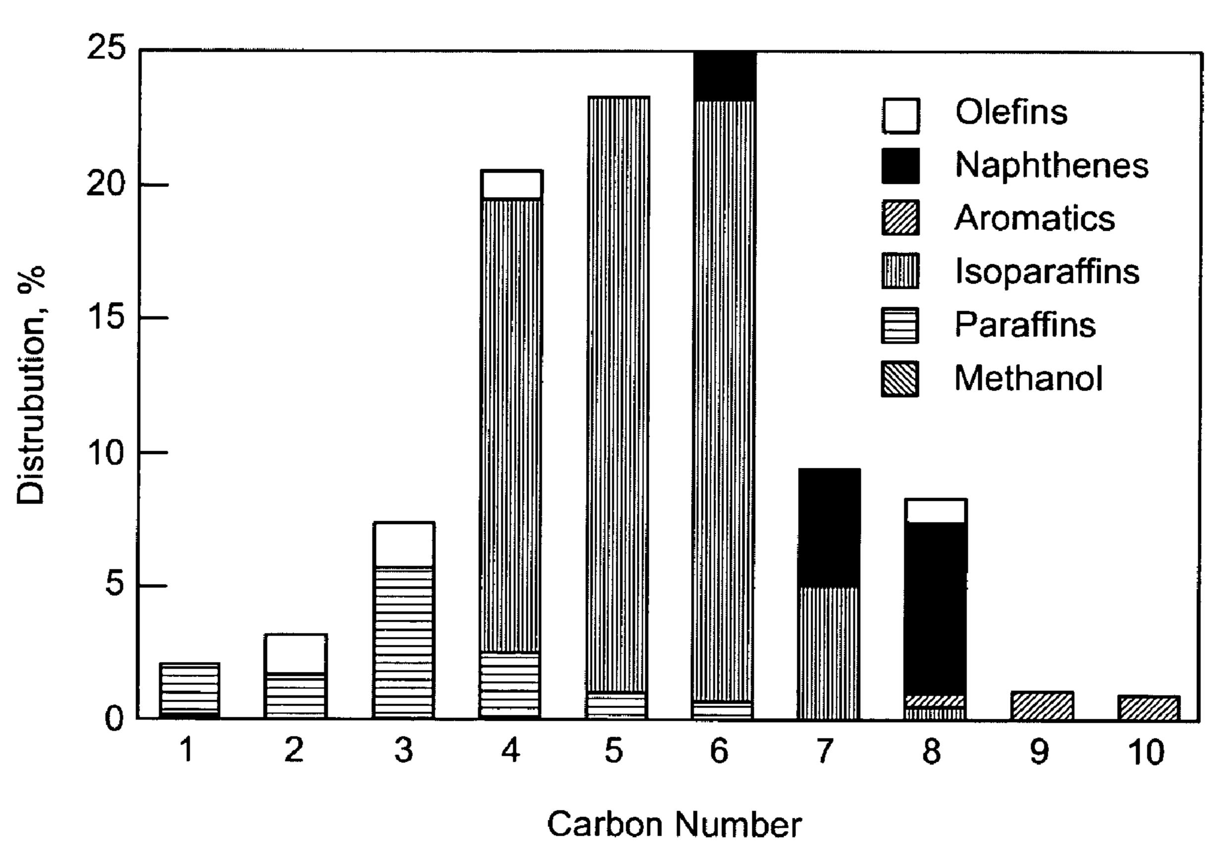
Figure 2 Syngas Conversion on  $2\text{ZnO-Cr}_2\text{O}_3$  + GaZSM-5 350°C, 40 atm, H<sub>2</sub>/CO = 2, TOS = 450h, GHSV = 3200h<sup>-1</sup>
