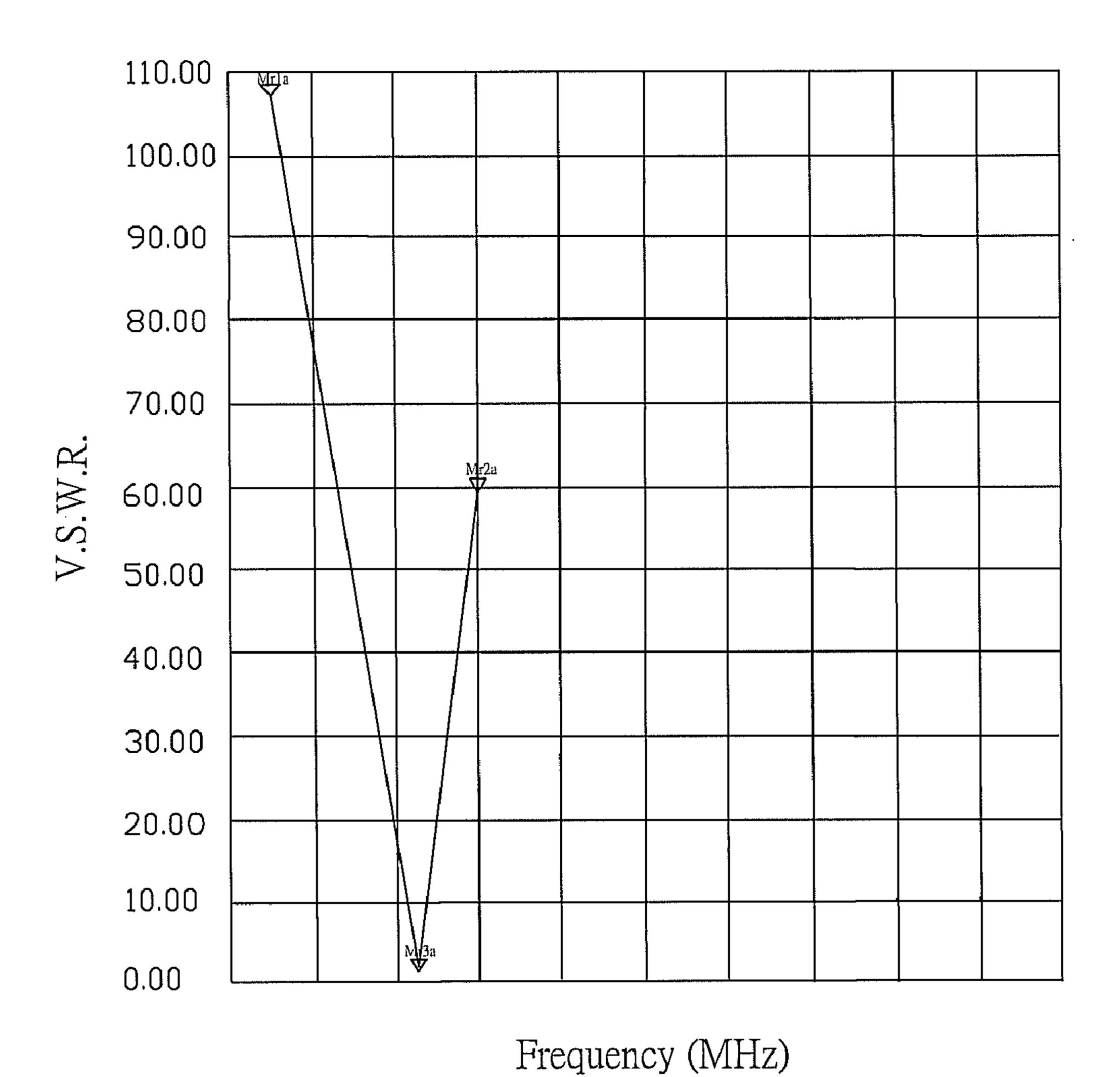
Mark1a 108.25 0.52MHz 59.486 1.71MHz Mark2a Mark3a 1.7801 1.334MHz
