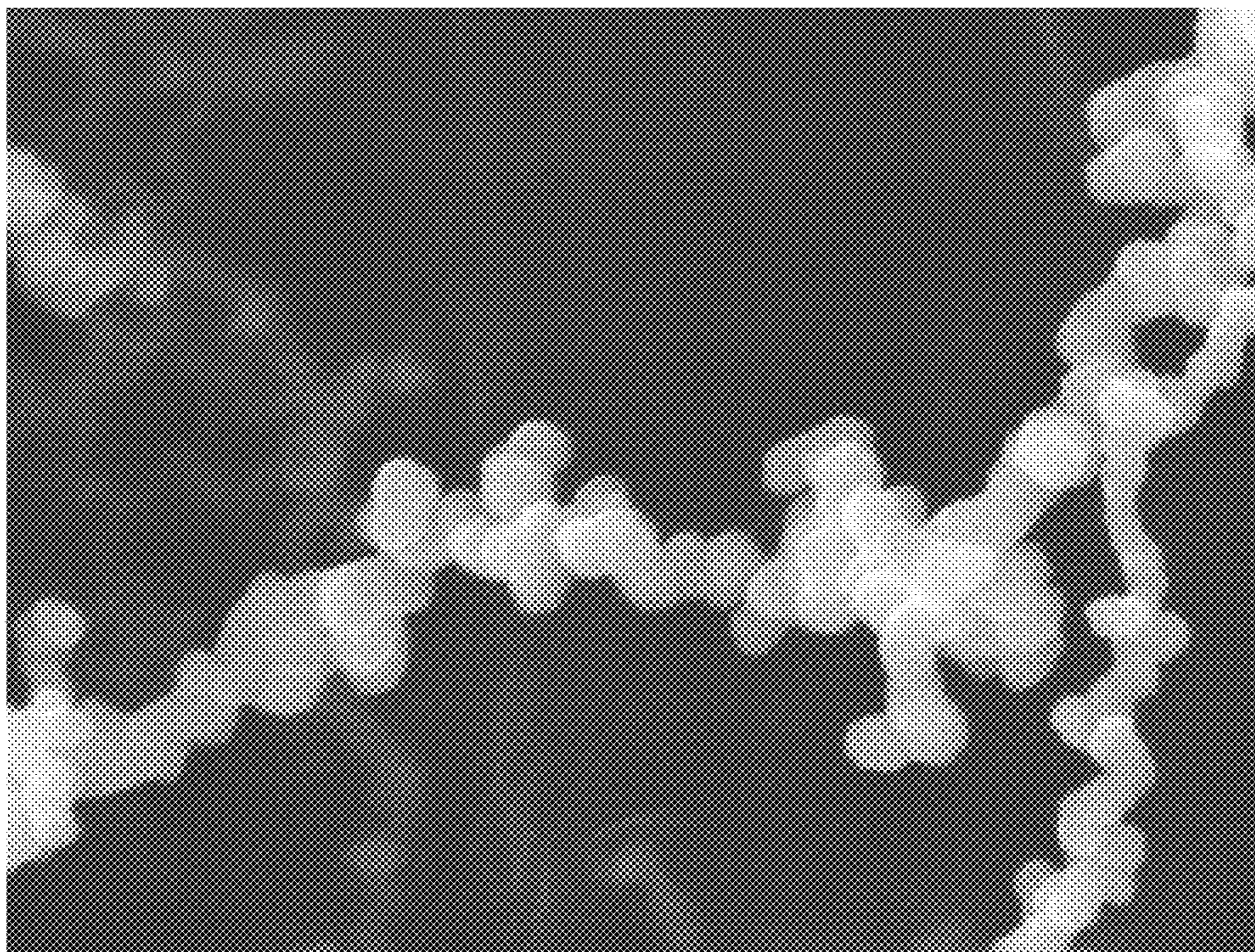
Nickel 70-nanometer branching nanostrands, enlarged 40,000 times
