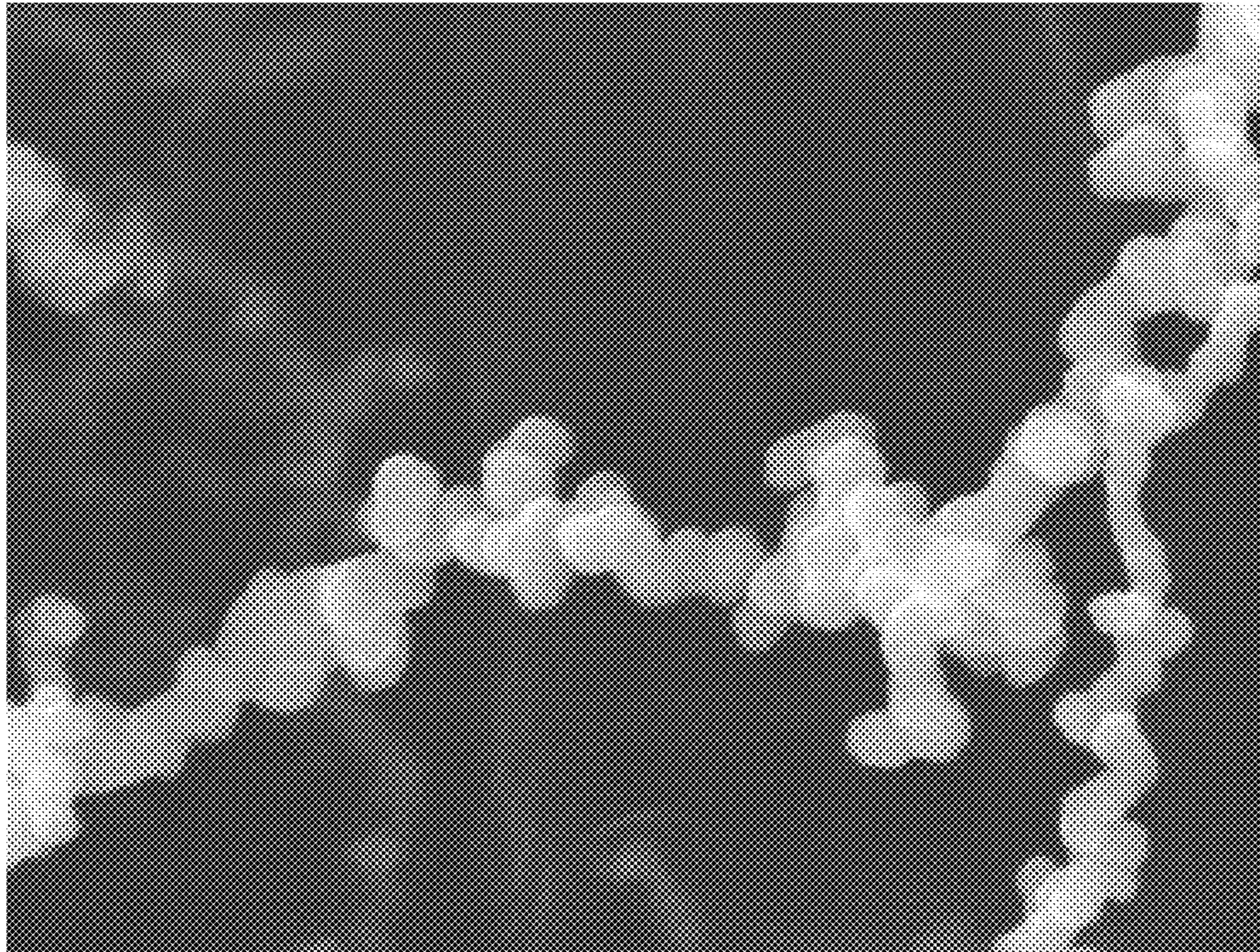
Nickel 70-nanometer branching nanostrands, enlarged 40,000 times
