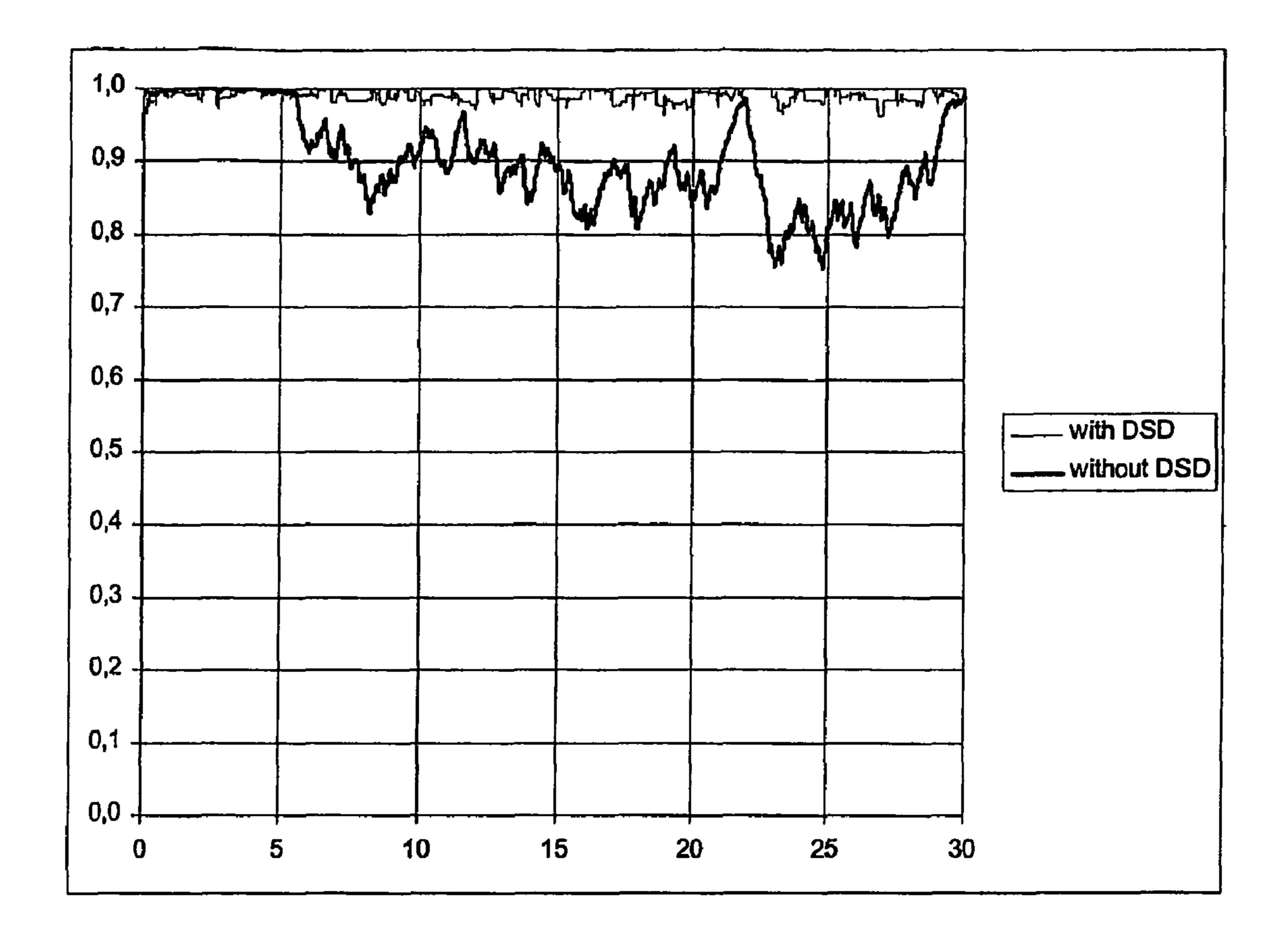
Omni parameter with and without DSD circuit
