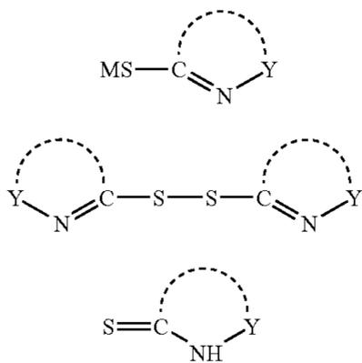
wherein: Y represents the non-metallic atoms needed to complete a saturated or unsaturated 5- or 6-membered heterocyclic nucleus, which may carry a fused-on aromatic ring system, and M represents hydrogen, an alkali metal atom, a quaternary ammonium group, or a negative charge forming an inner salt with a quaternized nitrogen atom of the heterocyclic compound.
