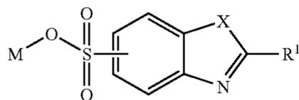
wherein M is hydrogen, an alkali atom or an ammonium group; R<sup>1</sup> is an alkyl, alkenyl-, alkynyl-, thioalkyl-, thioalkenyl- or thioalkynyl-group in which the alkyl-, alkenyl- or alkynyl-group has 6 to 25 carbon atoms; X is —O—, —S— or —N(R<sup>2</sup>)—; and R<sup>2</sup> is hydrogen, a —(CH<sub>2</sub>)<sub>m</sub>SO<sub>3</sub>M group or a
