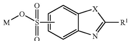
wherein M is hydrogen, an alkali atom or an ammonium group; R<sup>1</sup> is an alkyl, alkenyl-, alkynyl-, thioalkyl-, thioalkenyl- or thioalkynyl-group in which the alkyl-, alkenyl- or alkynyl-group has 6 to 25 carbon atoms; X is —O—, —S— or —N(R<sup>2</sup>)—; and R<sup>2</sup> is hydrogen, a
