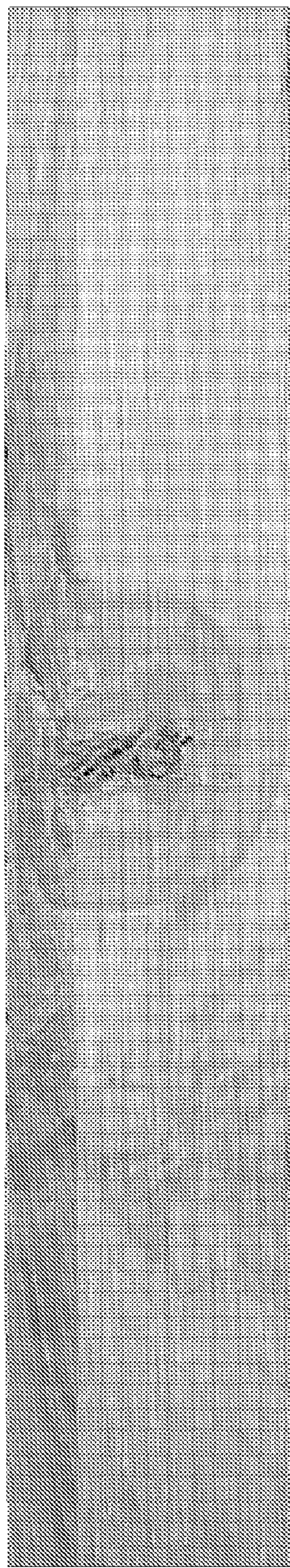
FIG. 5c : Stick with a knot defect
