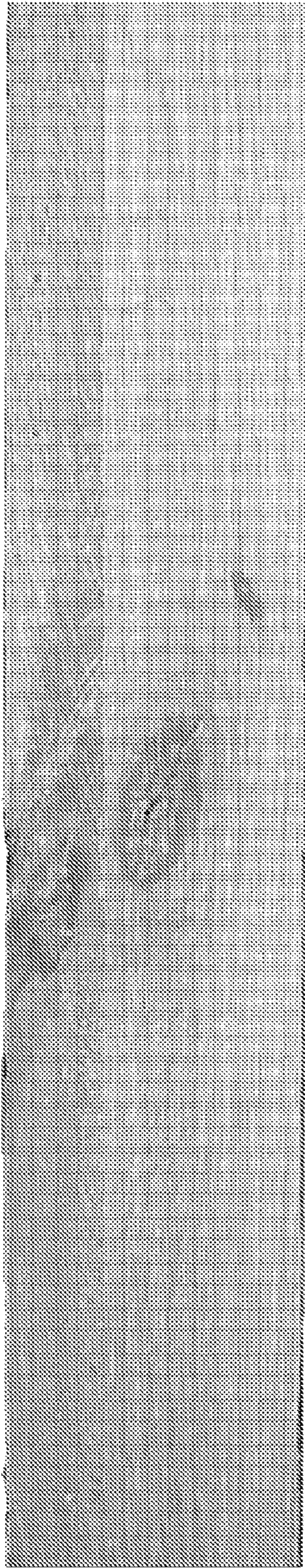
FIG. 5b : Stick with a knot defect
