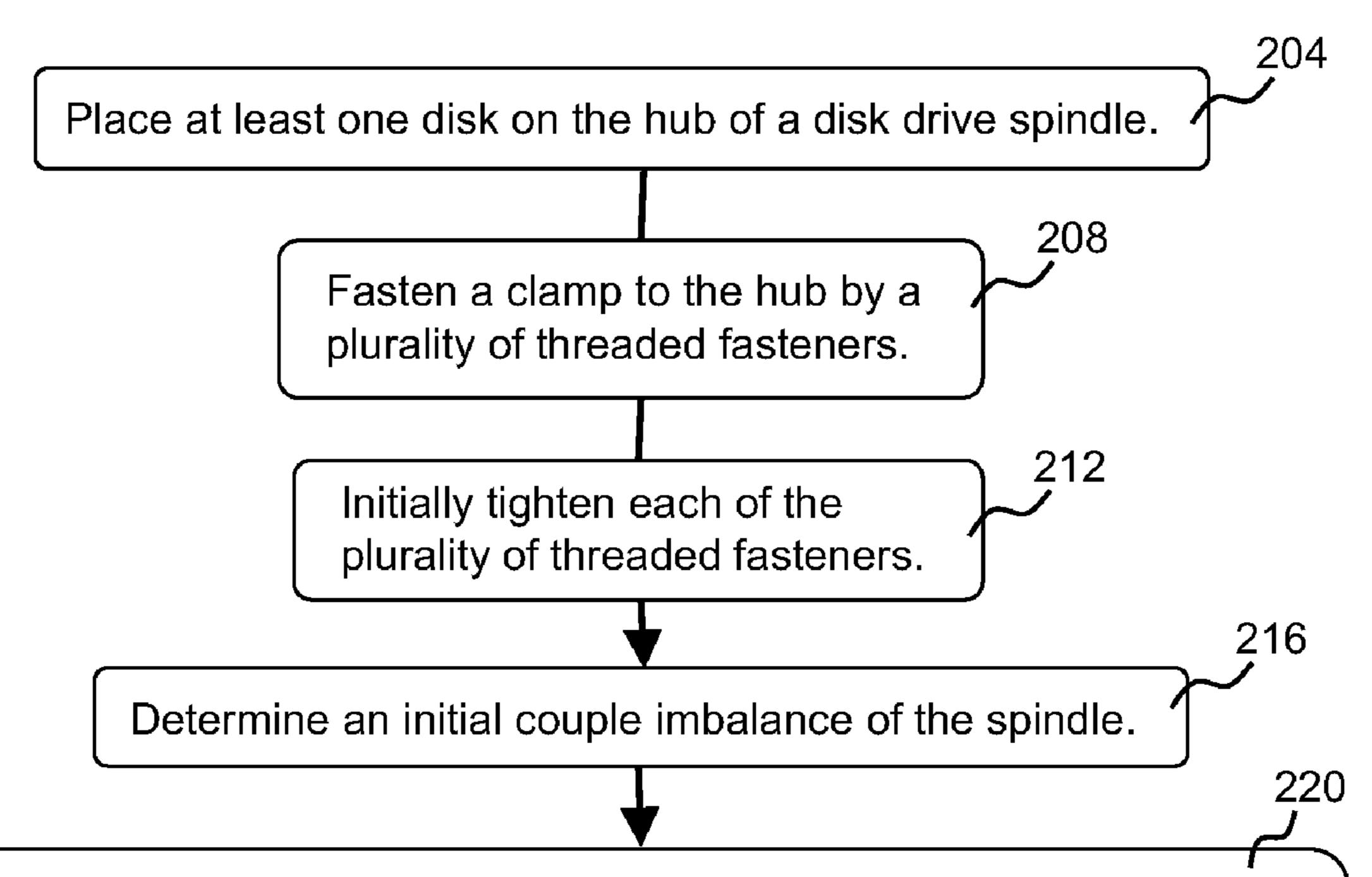
Based on the initial couple imbalance of the spindle, select and rotate a first selected threaded fastener of the plurality of threaded fasteners by a first amount of rotation that is significantly different from a second amount of rotation of a second selected threaded fastener of the plurality of threaded fasteners.
