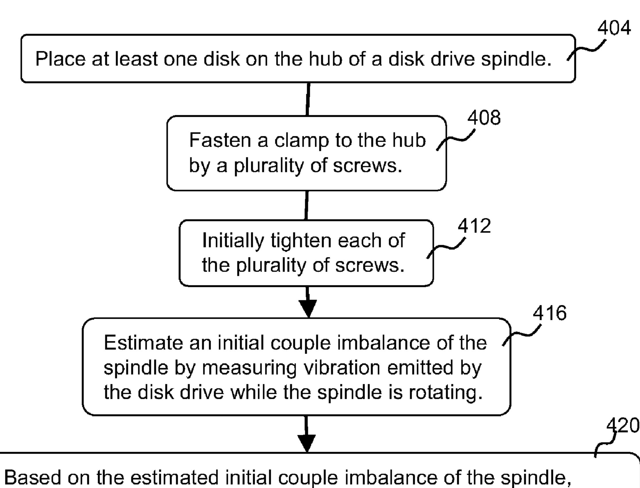
torque a first selected screw of the plurality of screws significantly differently than a second selected screw of the plurality of screws.
