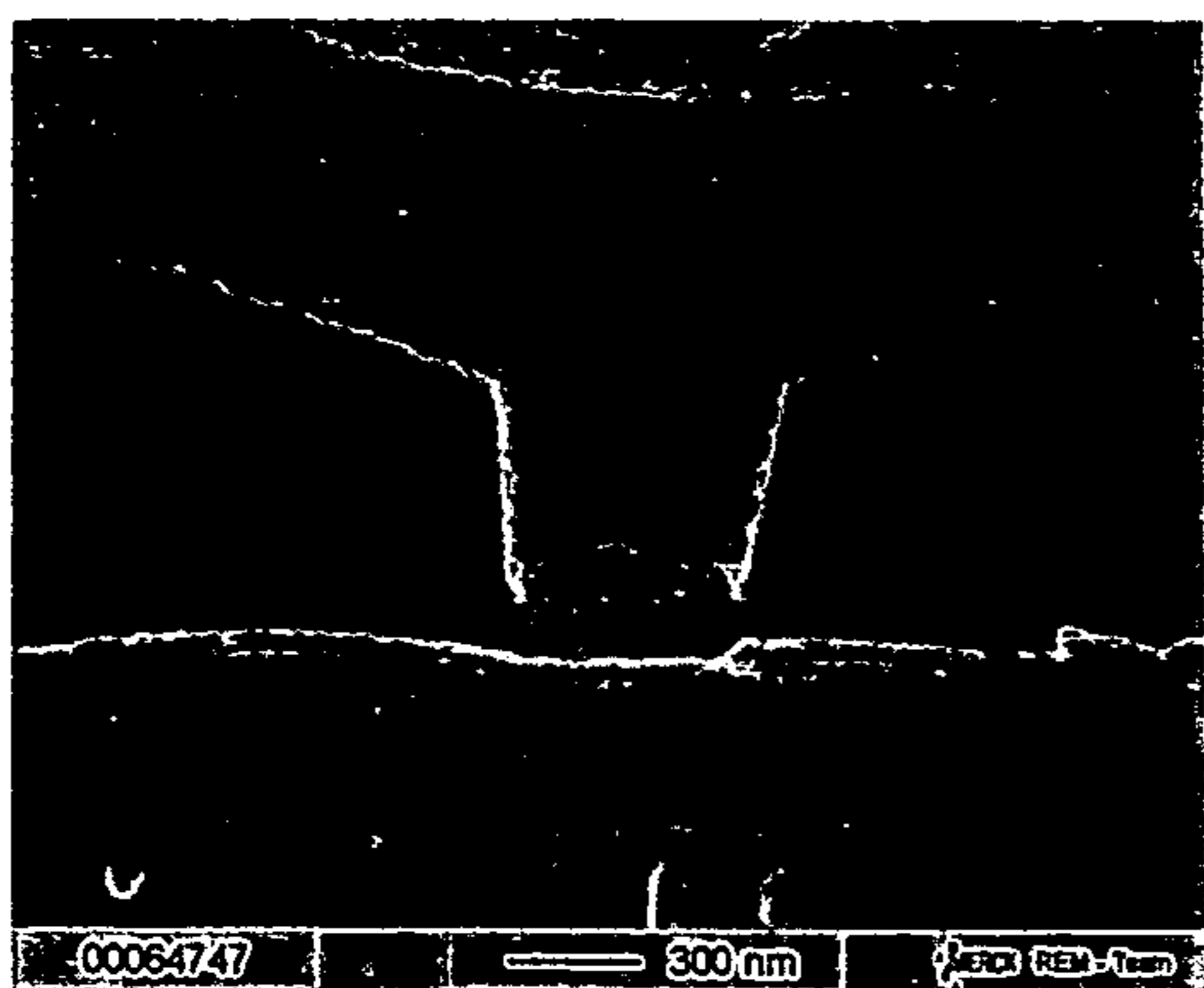
Figure 10: After cleaning for 20 min at 60°C with maleic acid 5% / NMP 1% / enanthic acid 1000 ppm
