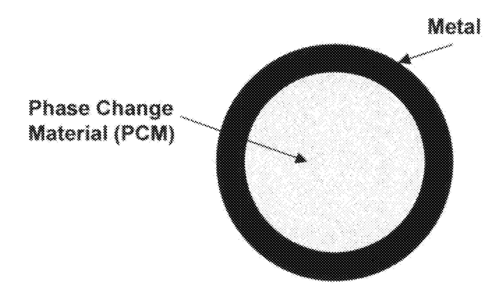
Structure of a PCM and metal shell hybrid nanoparticle
