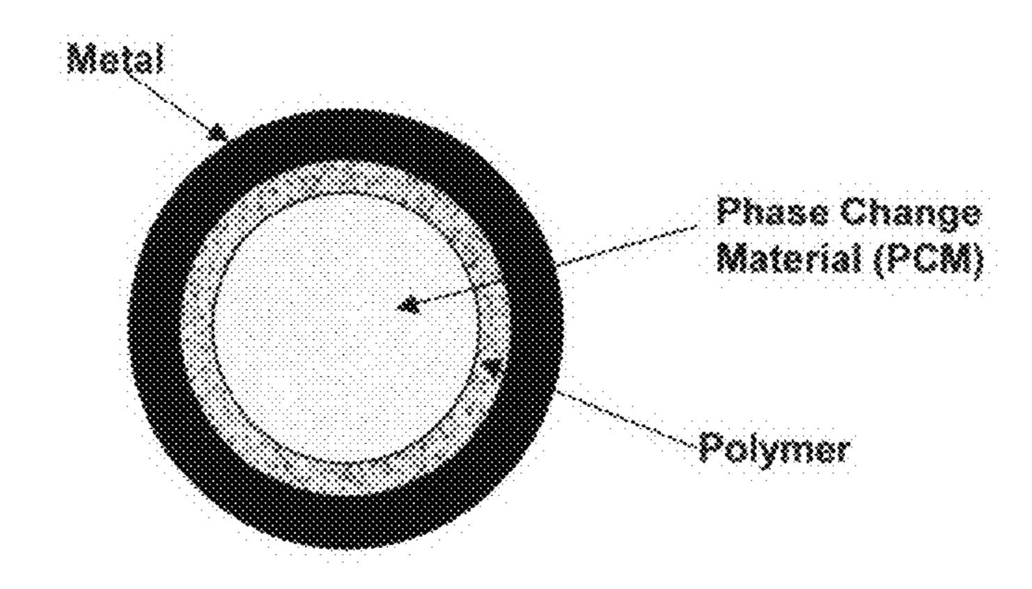
Figure 2. Structure of a PCM, polymer layer, and metal shell hybrid nanoparticle
