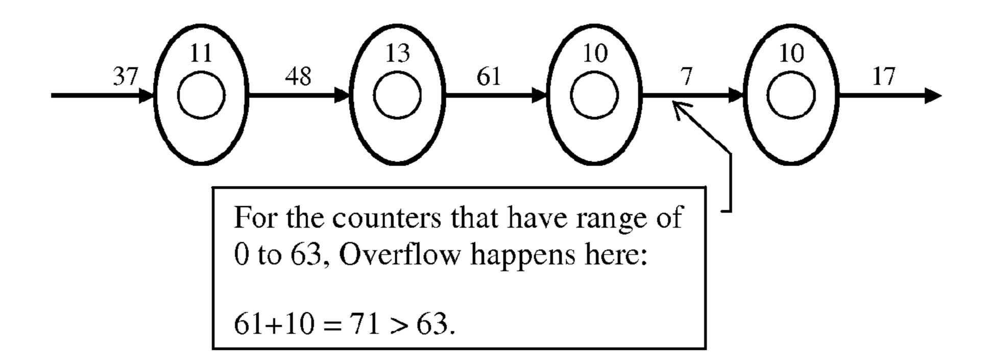
An example of the solution of the overflow situation of the system power number in the ring.
