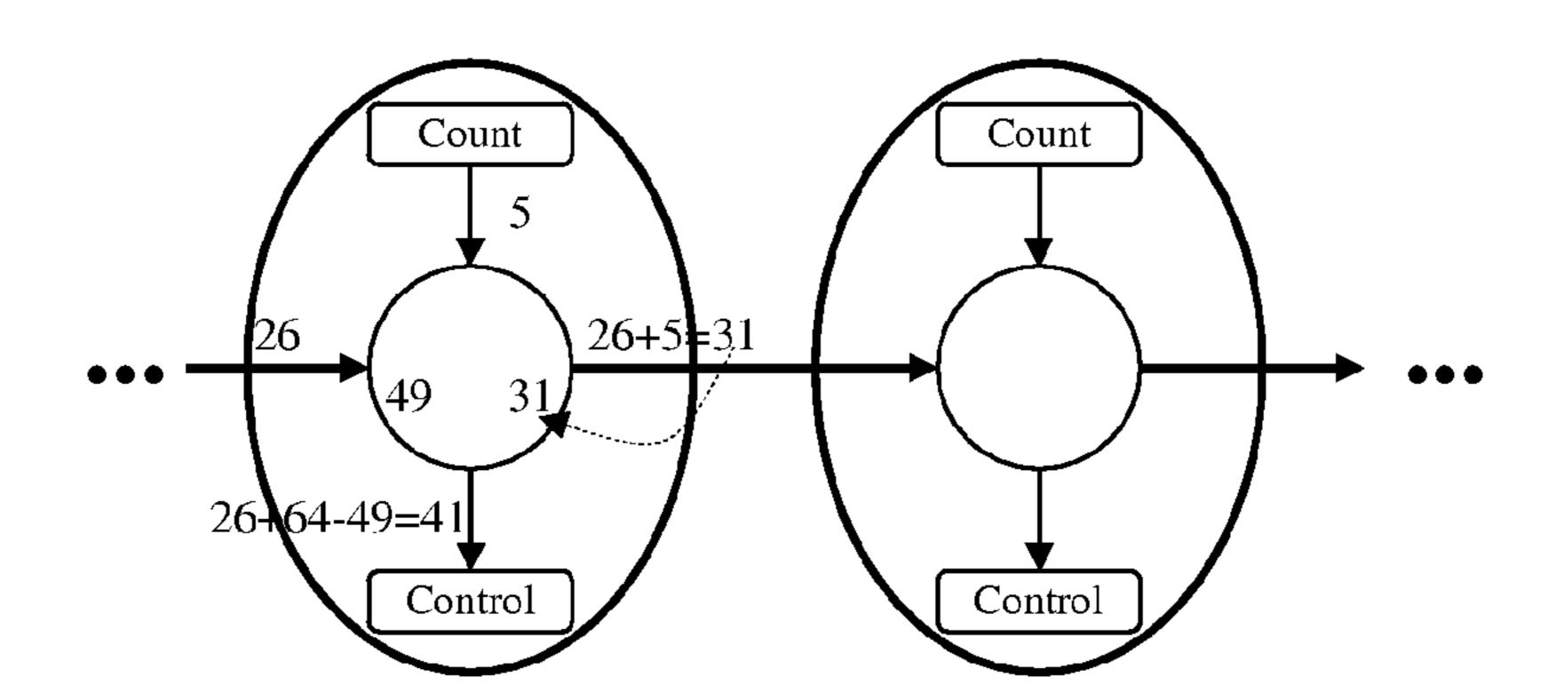
Single-number transfer mode versus multiple-transfer mode.
