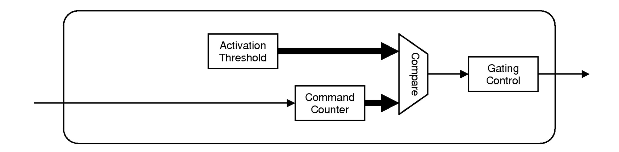
An example of new power governor design in a multi-node system. A closed ring is implemented.
