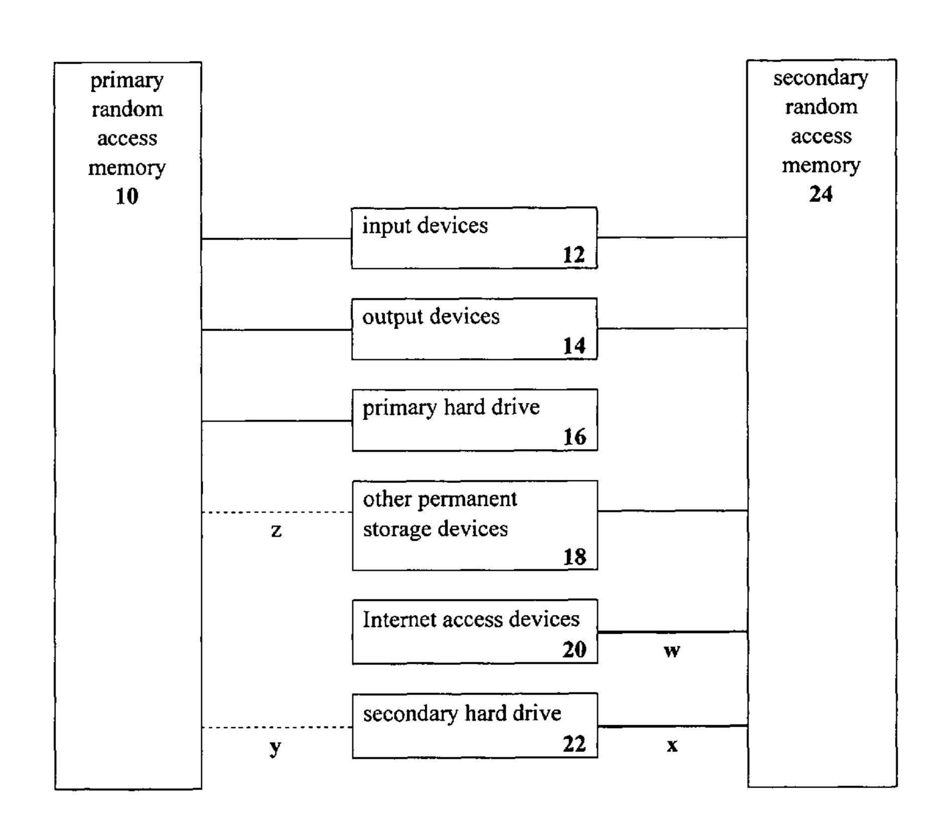
Figure 1A: Schematic of Present Invention
