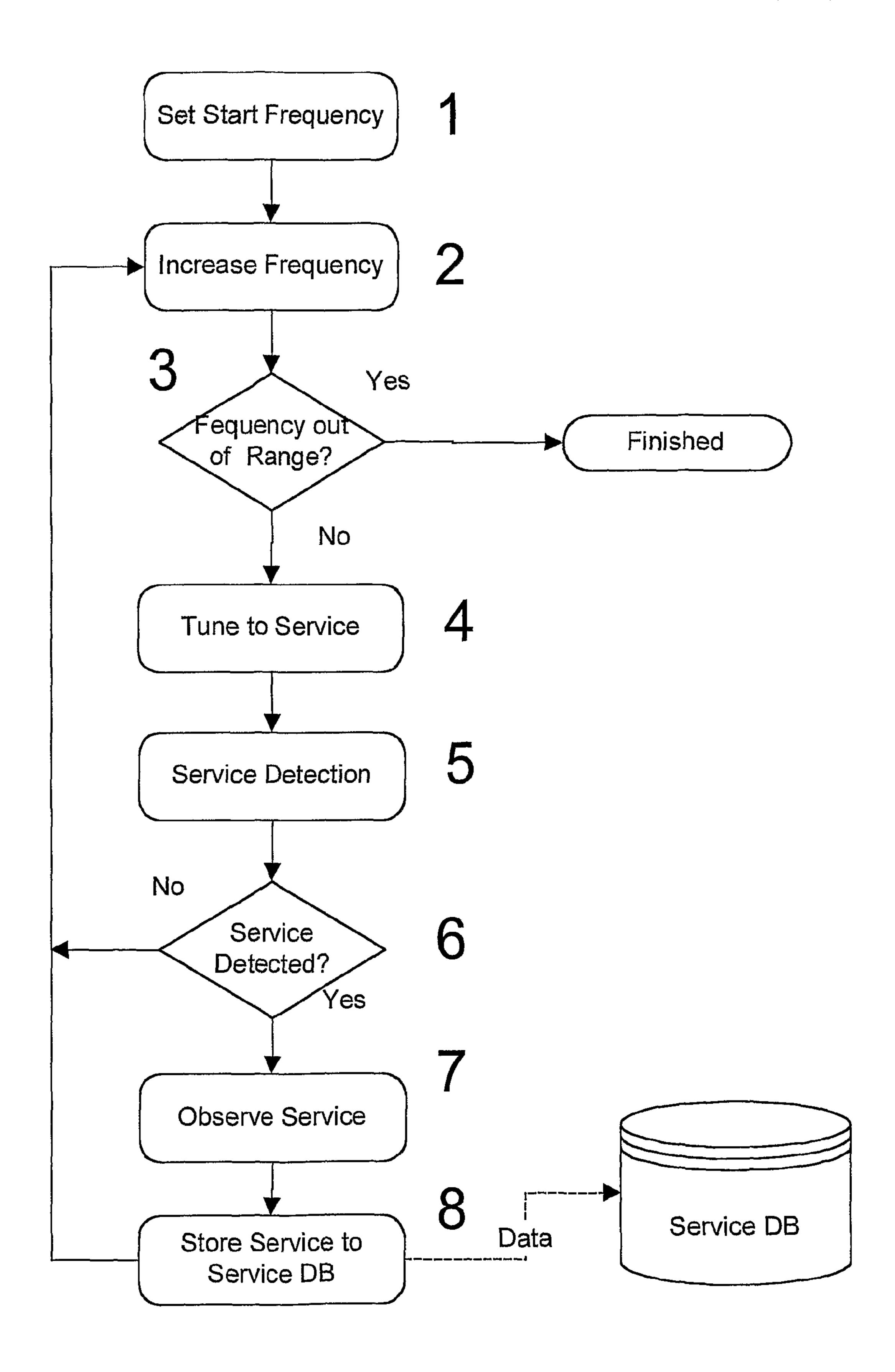
Fig. 3 - Conventional Tuning Process
