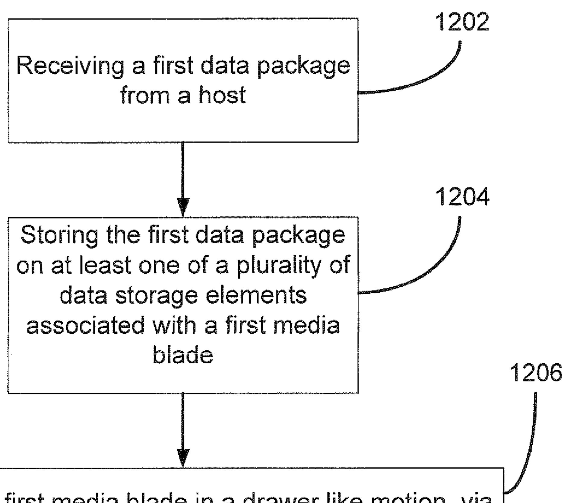
Moving the first media blade in a drawer like motion, via an accommodating opening in the cover, from between a first position, that is substantially within the interior space, and a second position, that is less than substantially within the interior space, while the storing step is being performed and without interrupting the storing step.
