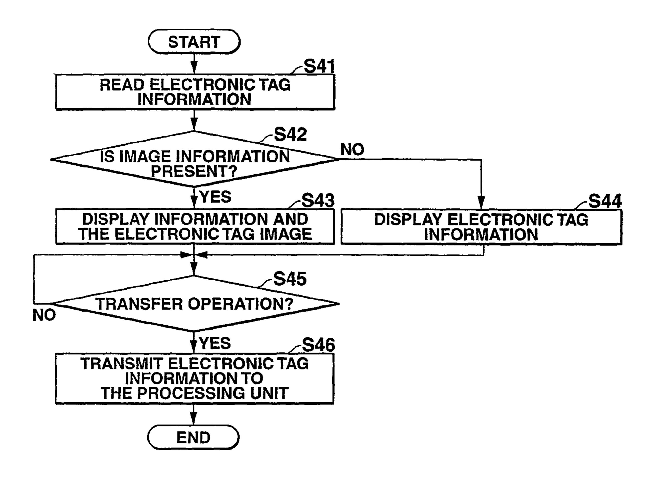
DIGITAL CAMERA INCLUDING AN ELECTRONIC TAG READER WHICH WIRELESSLY WRITES IMAGE DATA INTO AN ELECTRONIC TAG, SYSTEM INCLUDING THE DIGITAL CAMERA, ELECTRONIC TAG READING APPARATUS WHICH READS DATA INCLUDING IMAGE DATA FROM AN ELECTRONIC TAG, ELECTRONIC TAG READ/WRITE METHOD FOR A DIGITAL CAMERA AND ELECTRONIC TAG READING METHOD FOR AN ELECTRONIC TAG READING READER
