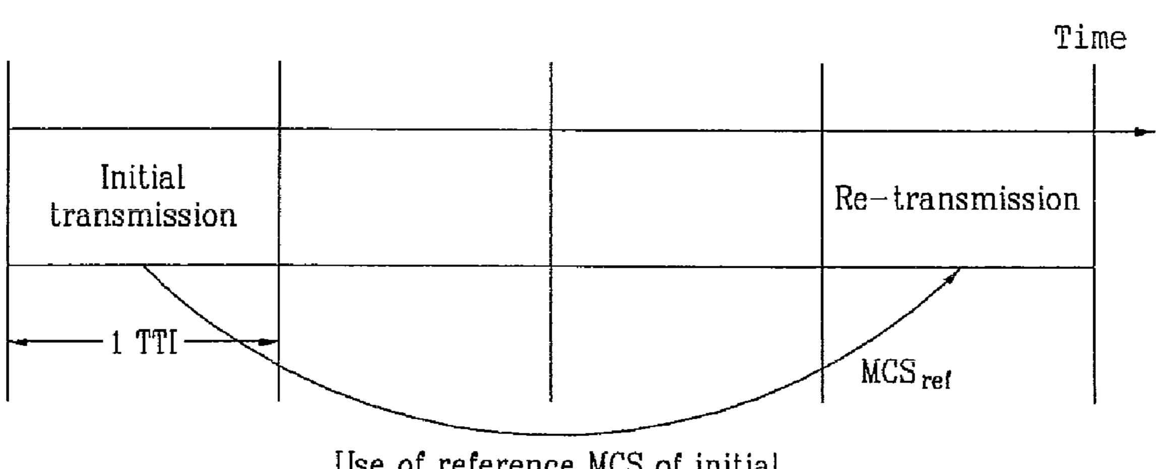
Use of reference MCS of initial transmission during re-transmission
