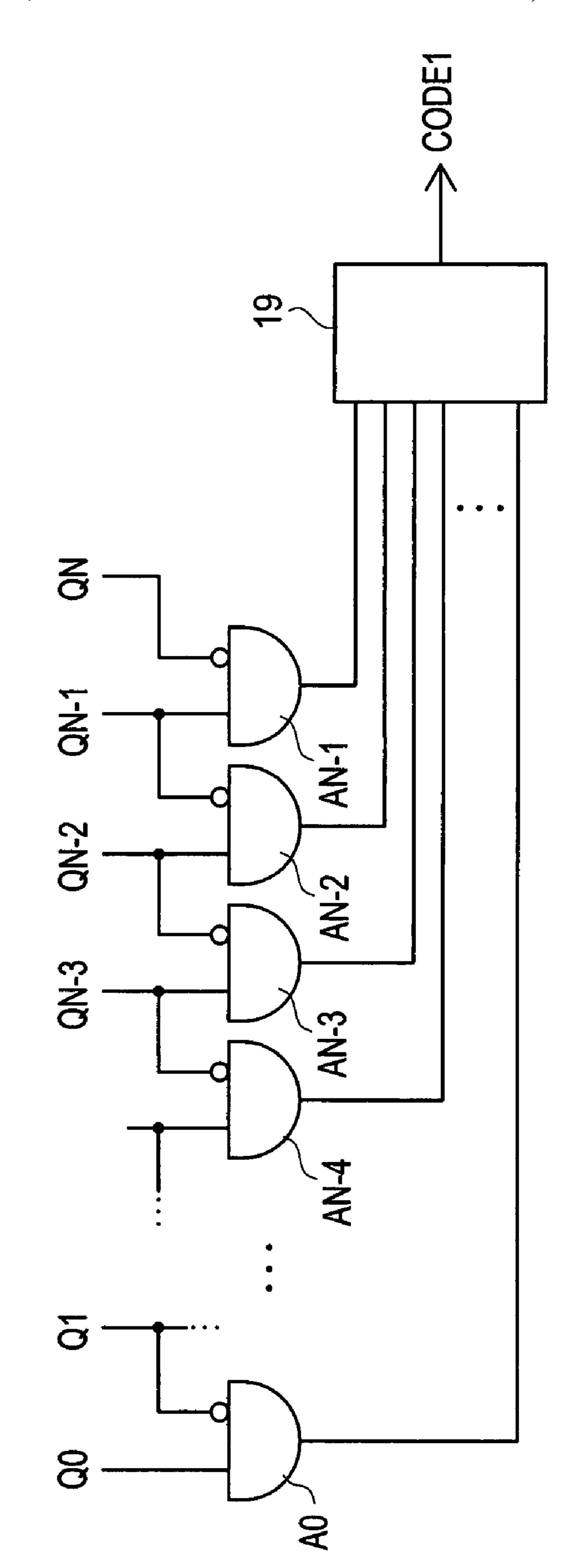
DIAGRAM SHOWING STRUCTURE OF DATA FETCH CIRCL ACCORDING TO THIRD EMBODIMENT
