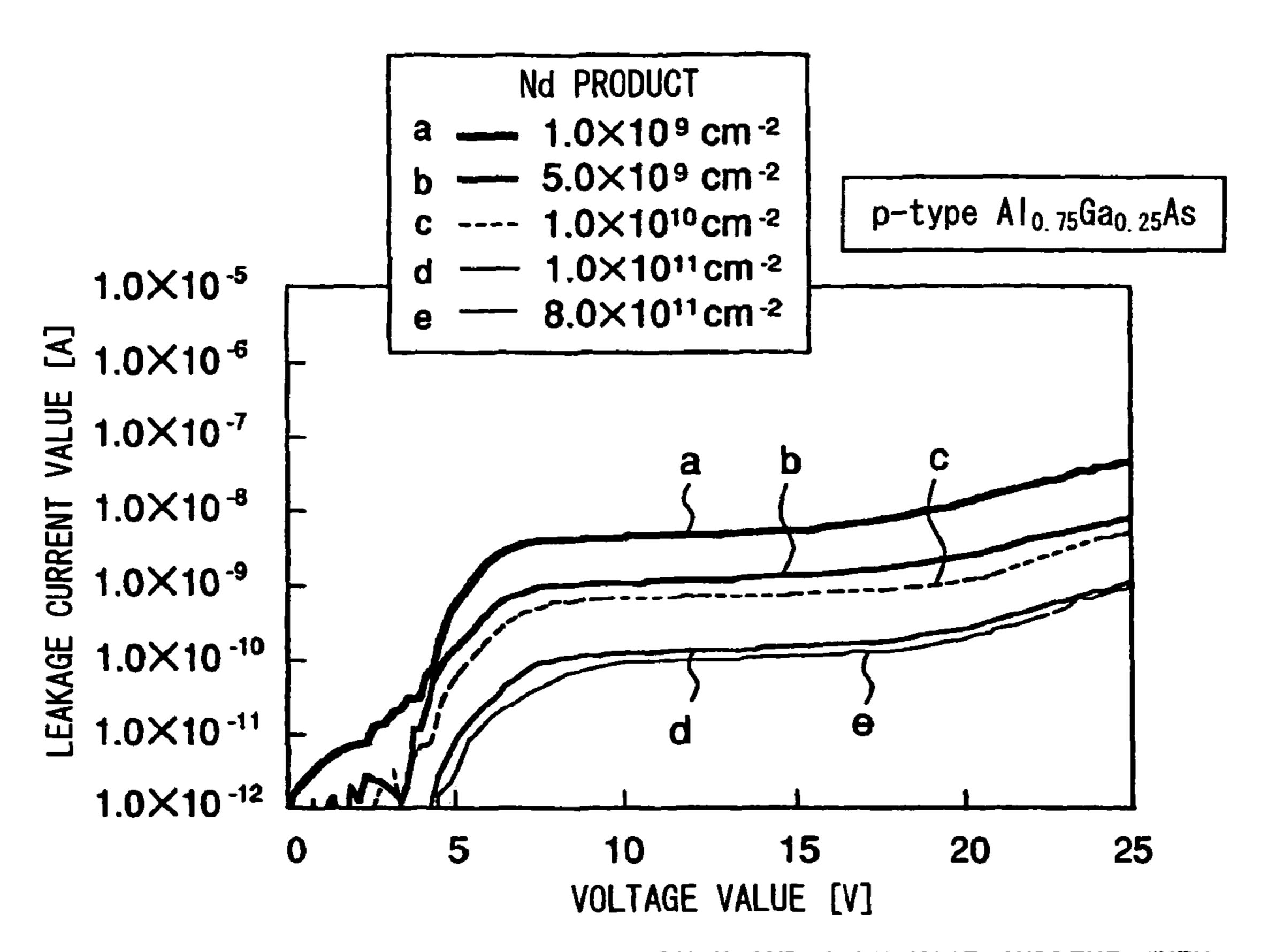
(RELATIONSHIP BETWEEN A Nd PRODUCT AND A LEAKAGE CURRENT WHEN A VOLTAGE IS APPLIED WHEREIN A MIX CRYSTAL RATIO IS 0.75)
