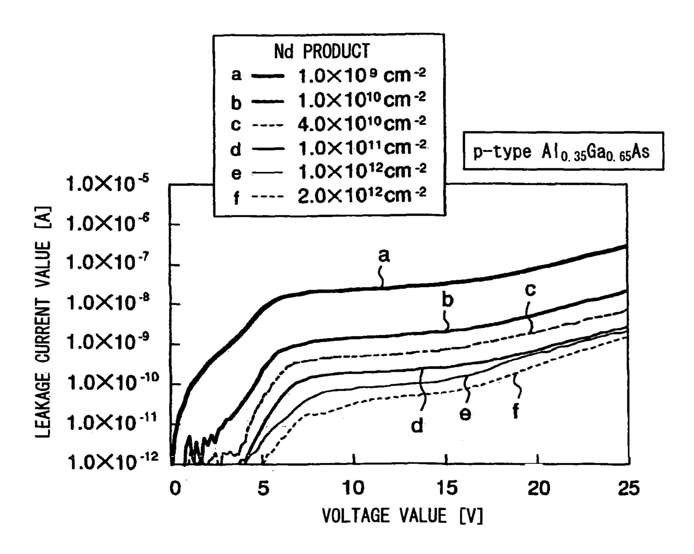
(RELATIONSHIP BETWEEN A Nd PRODUCT AND A LEAKAGE CURRENT WHEN A VOLTAGE IS APPLIED WHEREIN A MIX CRYSTAL RATIO IS 0.35)
