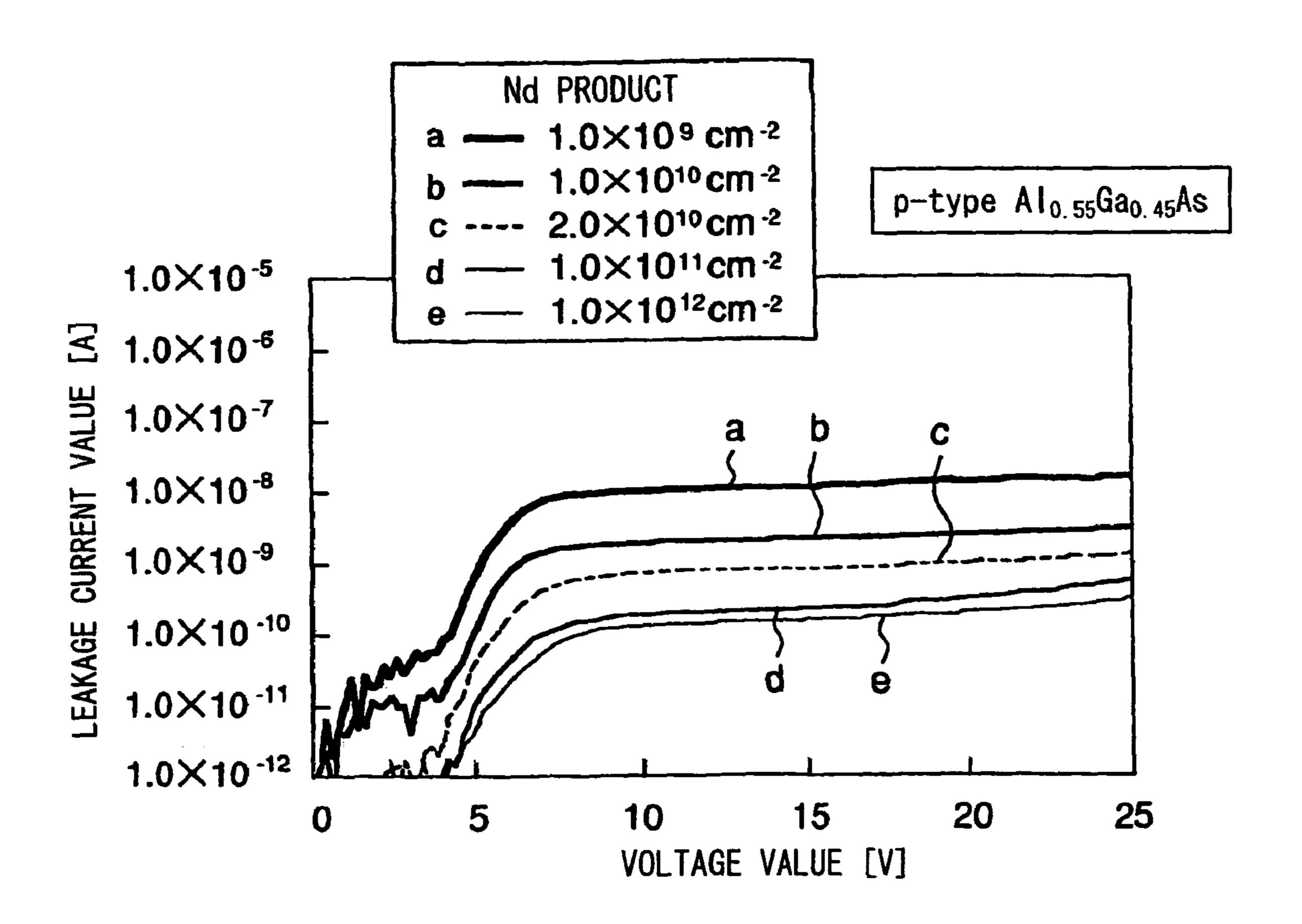
(RELATIONSHIP BETWEEN A Nd PRODUCT AND A LEAKAGE CURRENT WHEN A VOLTAGE IS APPLIED WHEREIN A MIX CRYSTAL RATIO IS 0.55)
