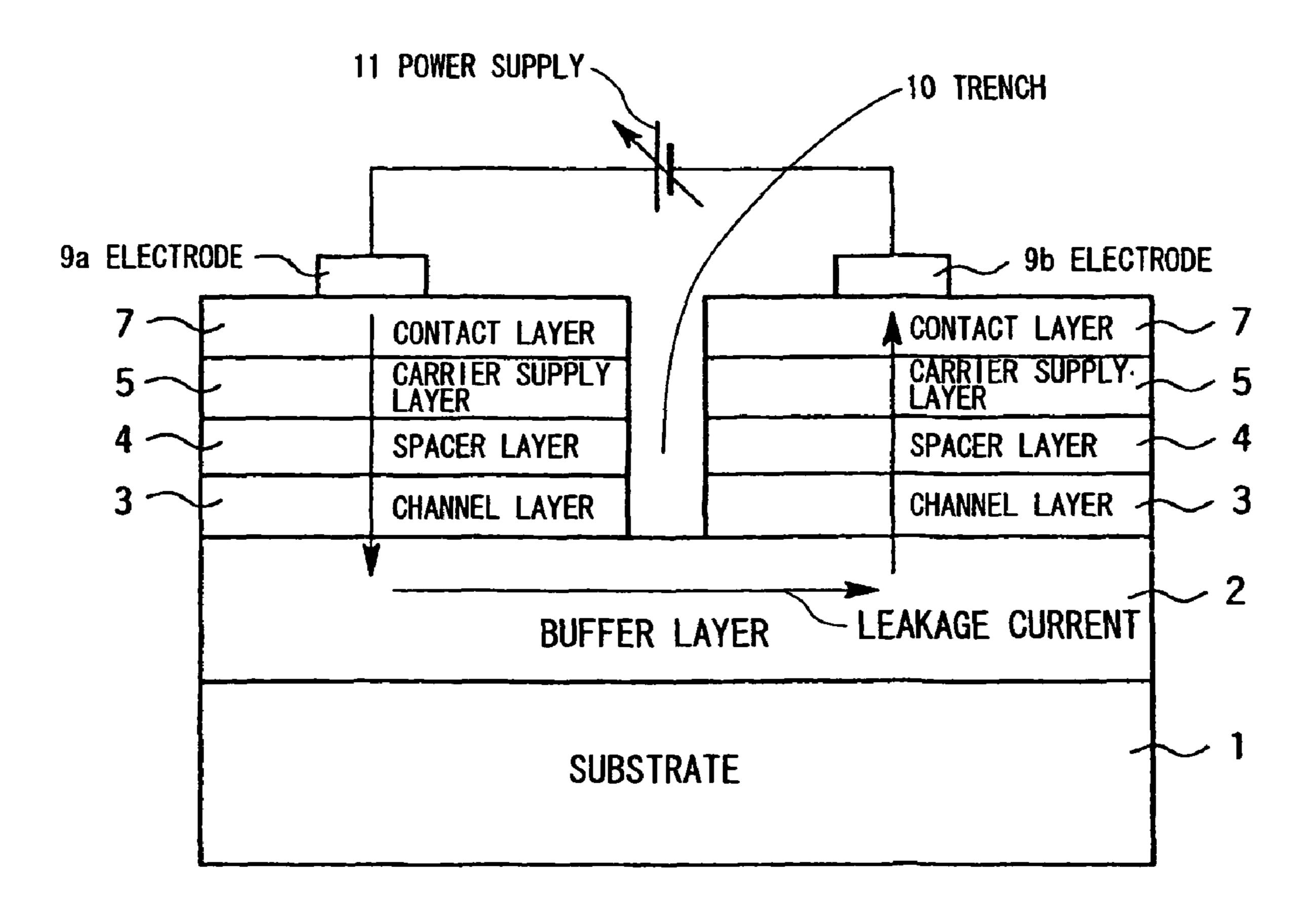
(METHOD OF MEASURING A LEAKAGE CURRENT IN A BUFFER LAYER WHEN A VOLTAGE IS APPLIED)
