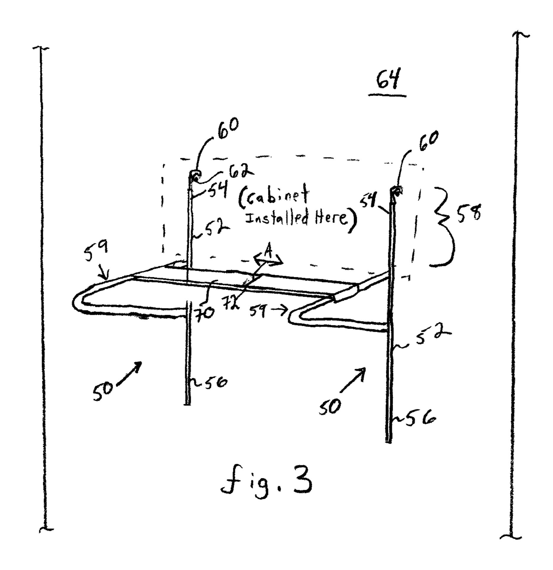
Place a jig upon a coupling device in or on a wall such that the jig is in a substantially vertical hanging position on the wall
