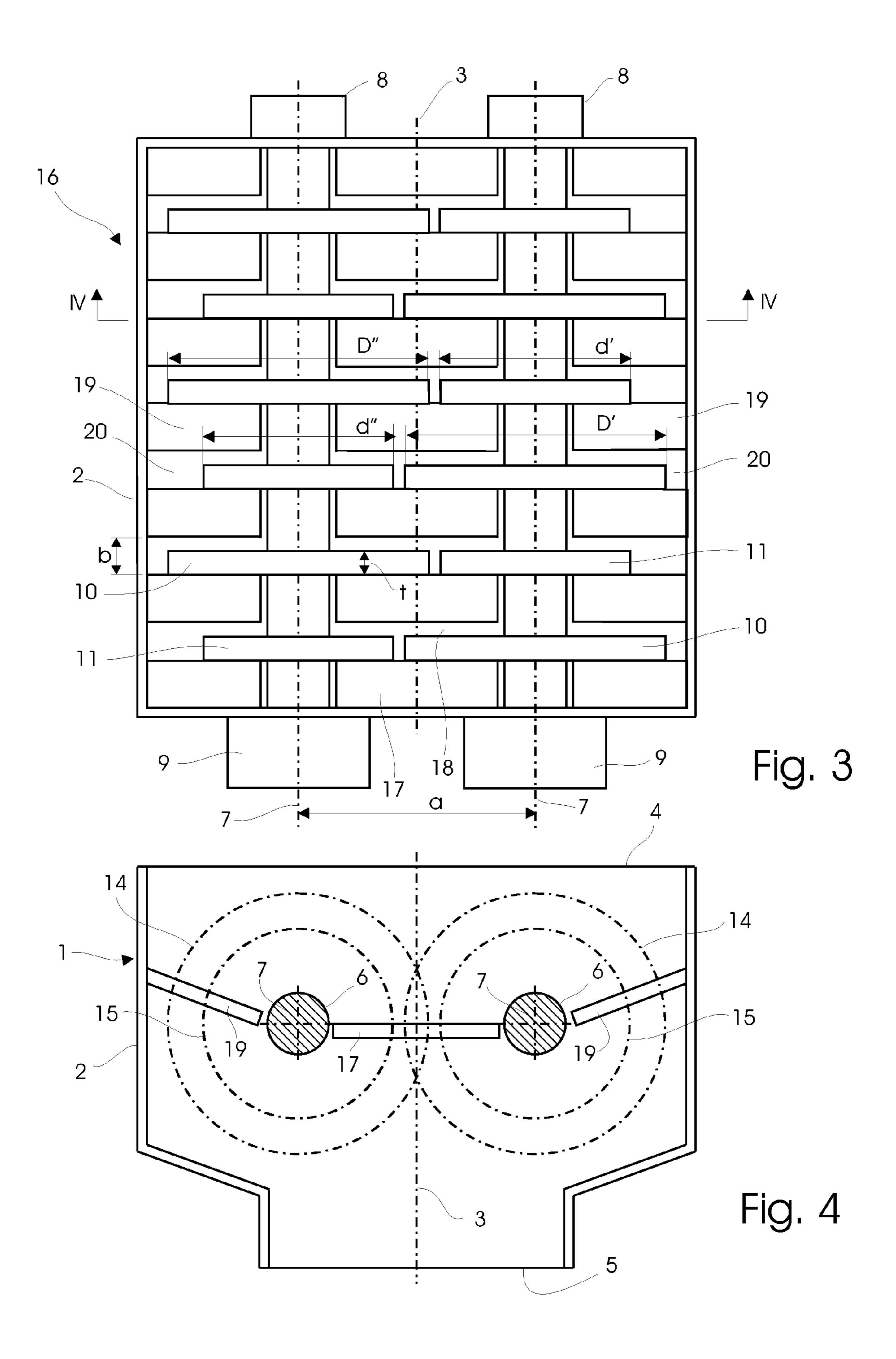
The invention relates to a comminution plant of the kind serving for comminution of materials and comprising at least one set of fixed bottom knifes separated by openings, at least two parallel shafts extending crosswise of the bottom knifes, a set of upper knifes attached on each shaft, the knifes are
