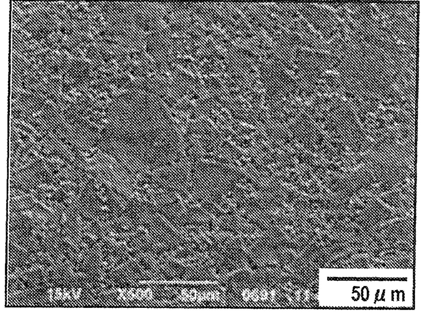
FIG.3 EXAMPLE 5 (KEEPING TEMPERATURE AT 850°C FOR 10 HOURS)
