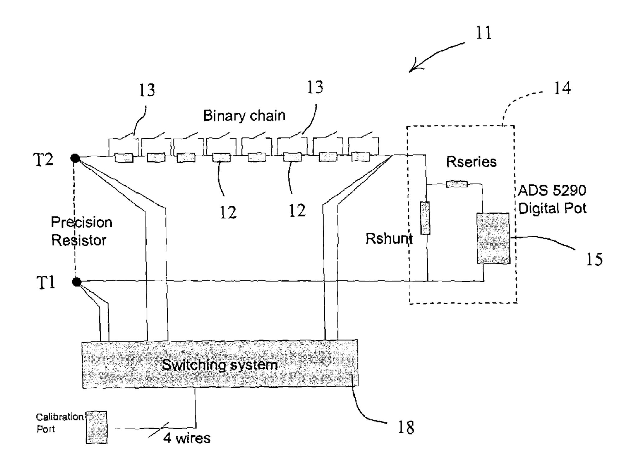
Precision Resistor using binary chain, digital potentiometer and a calibration port
