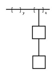
in which the continuous line is the main chain of the siloxane polymer and the squares represent the groups capable of establishing hydrogen interactions.
