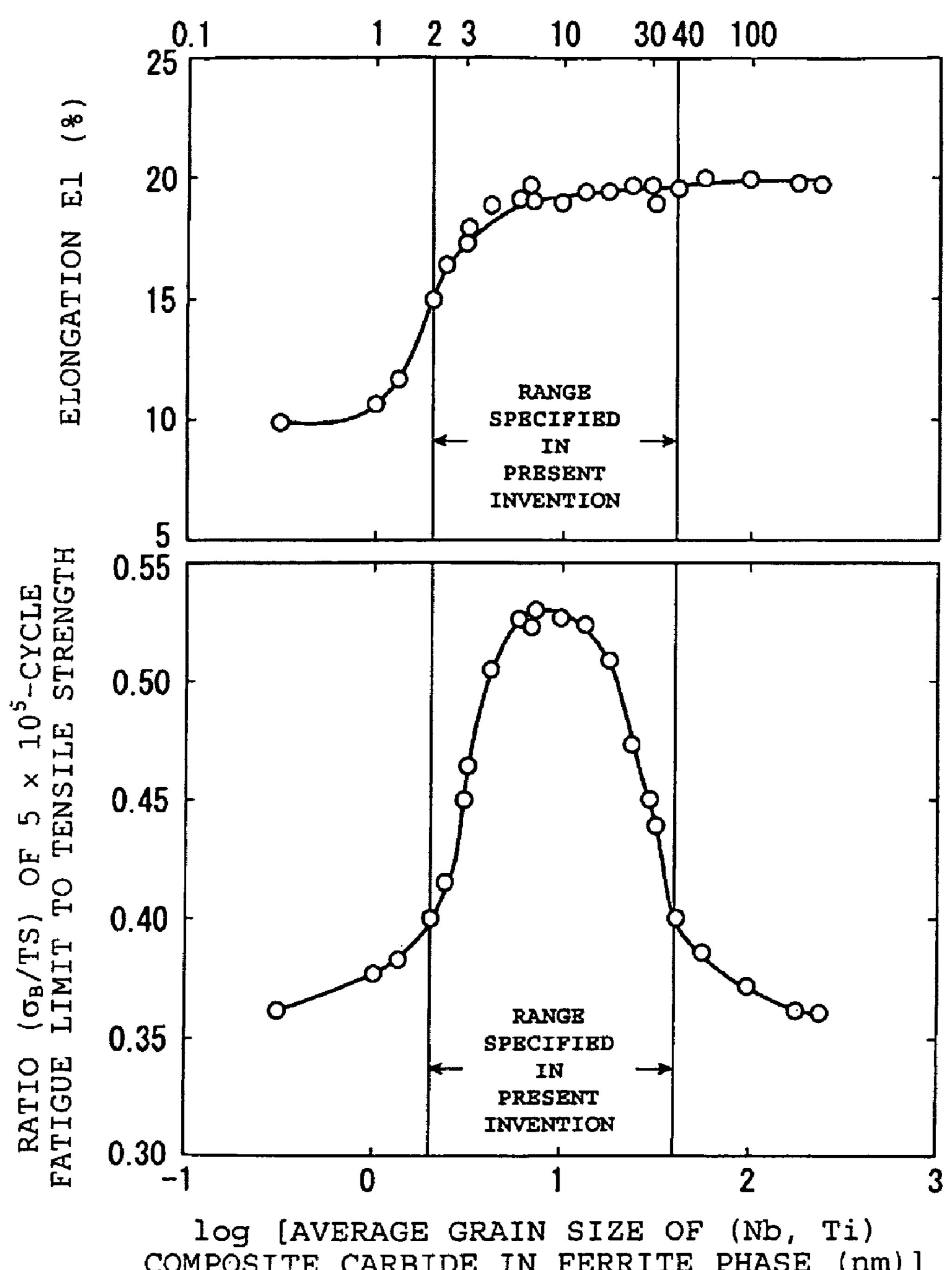
COMPOSITE CARBIDE IN FERRITE PHASE (nm)]
