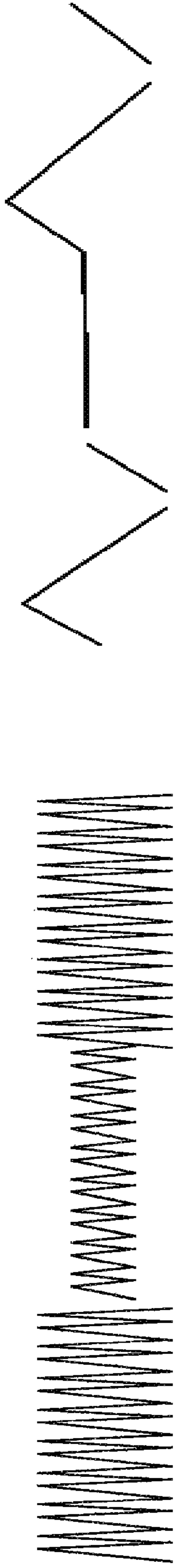
a) 4 Cycles per bit reduced amplitudes for 0 states b) Single cycle per bit with zero transmit for 0 State
