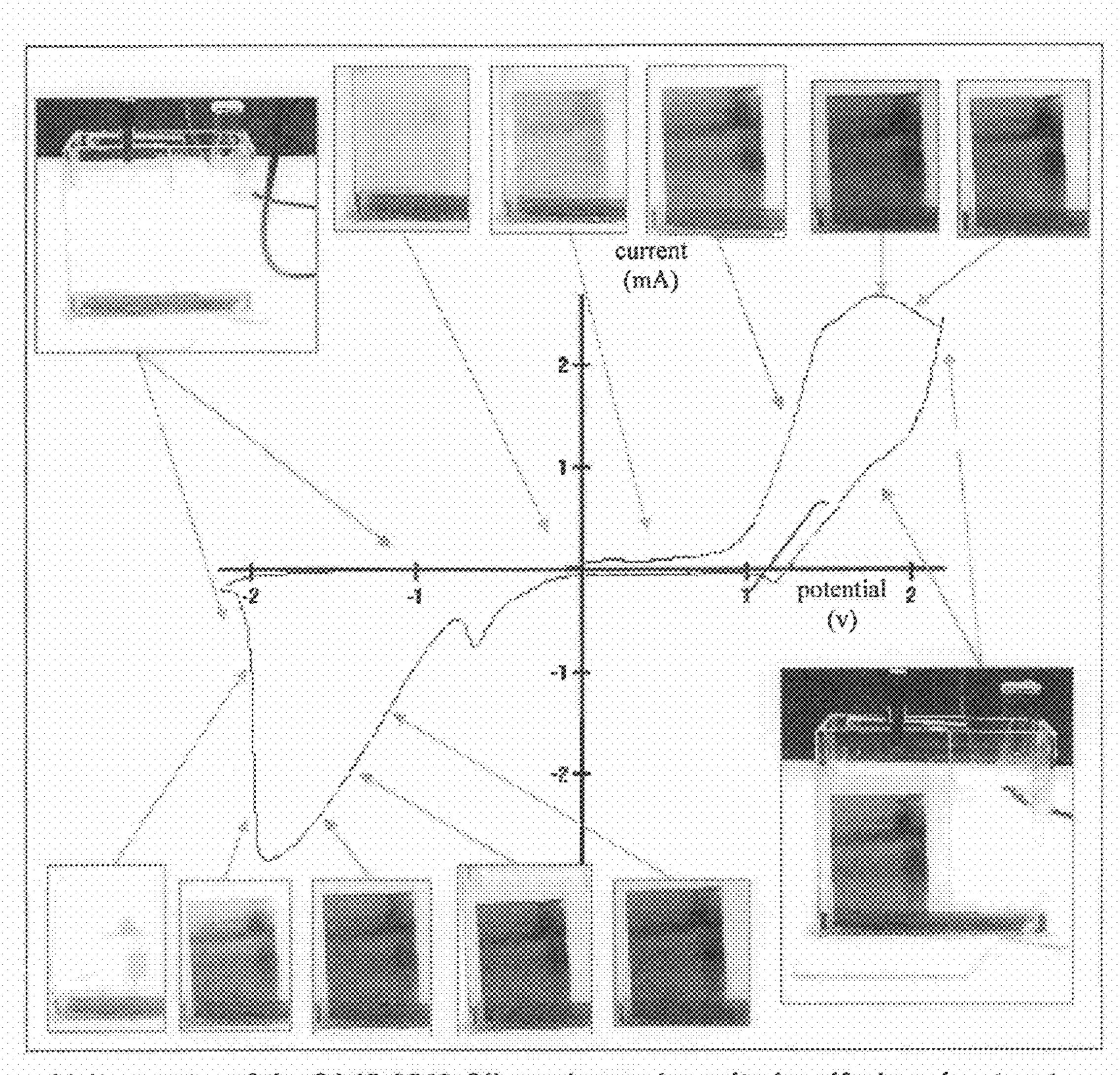
Voltammetry of the CA45-0549 Ciba polymer deposited on K-glass (cast wet thickness: 60 µm) – liquid electrolyte: 50/50 water/acetonitrile mixture with 0.5M LiClO4 (connection: bare K-glass = working electrode + reference electrode, K-glass + Ciba polymer = counterelectrode) – scan rate: 10 mV/s.
