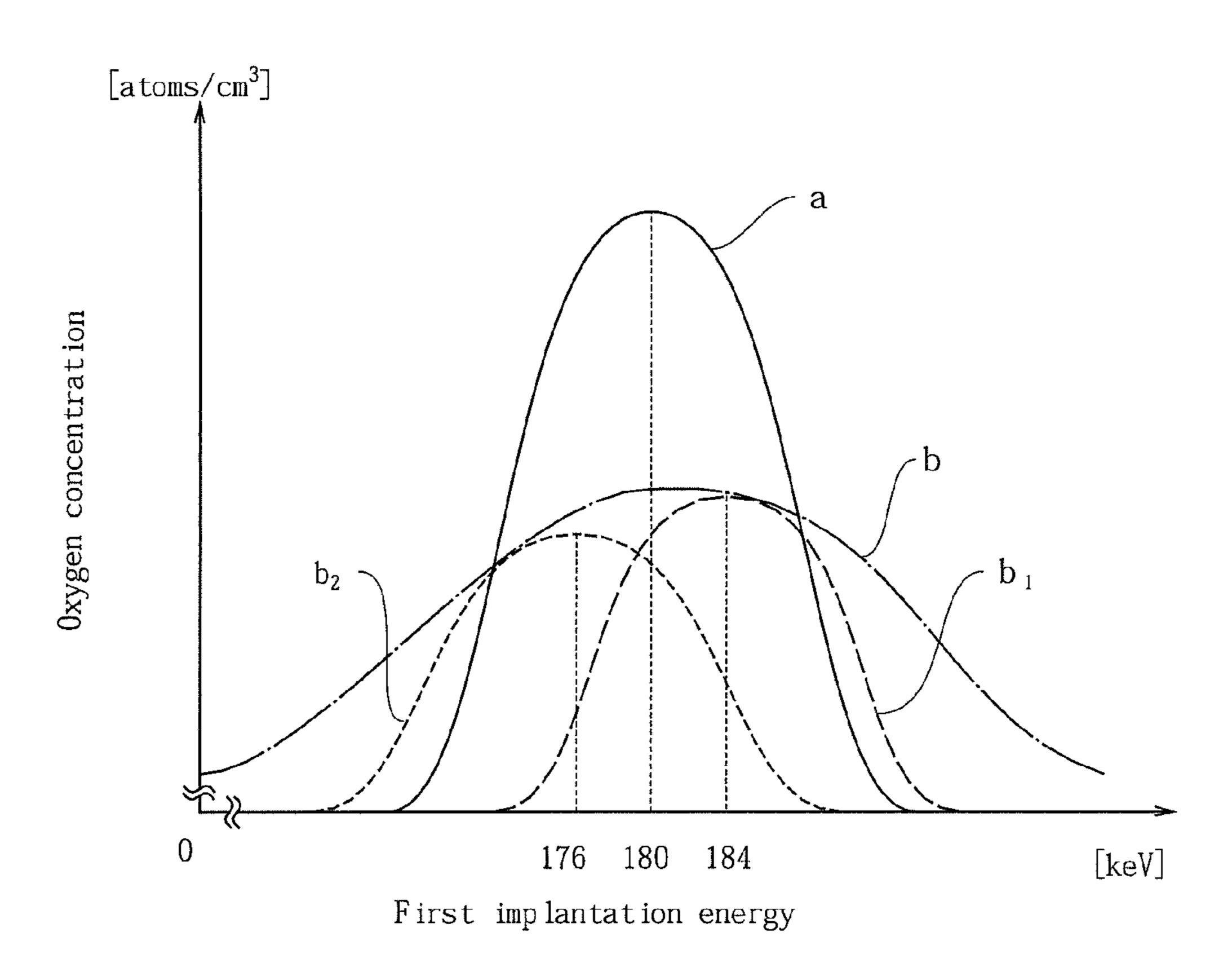
a : Ion implantation by single implatation step
