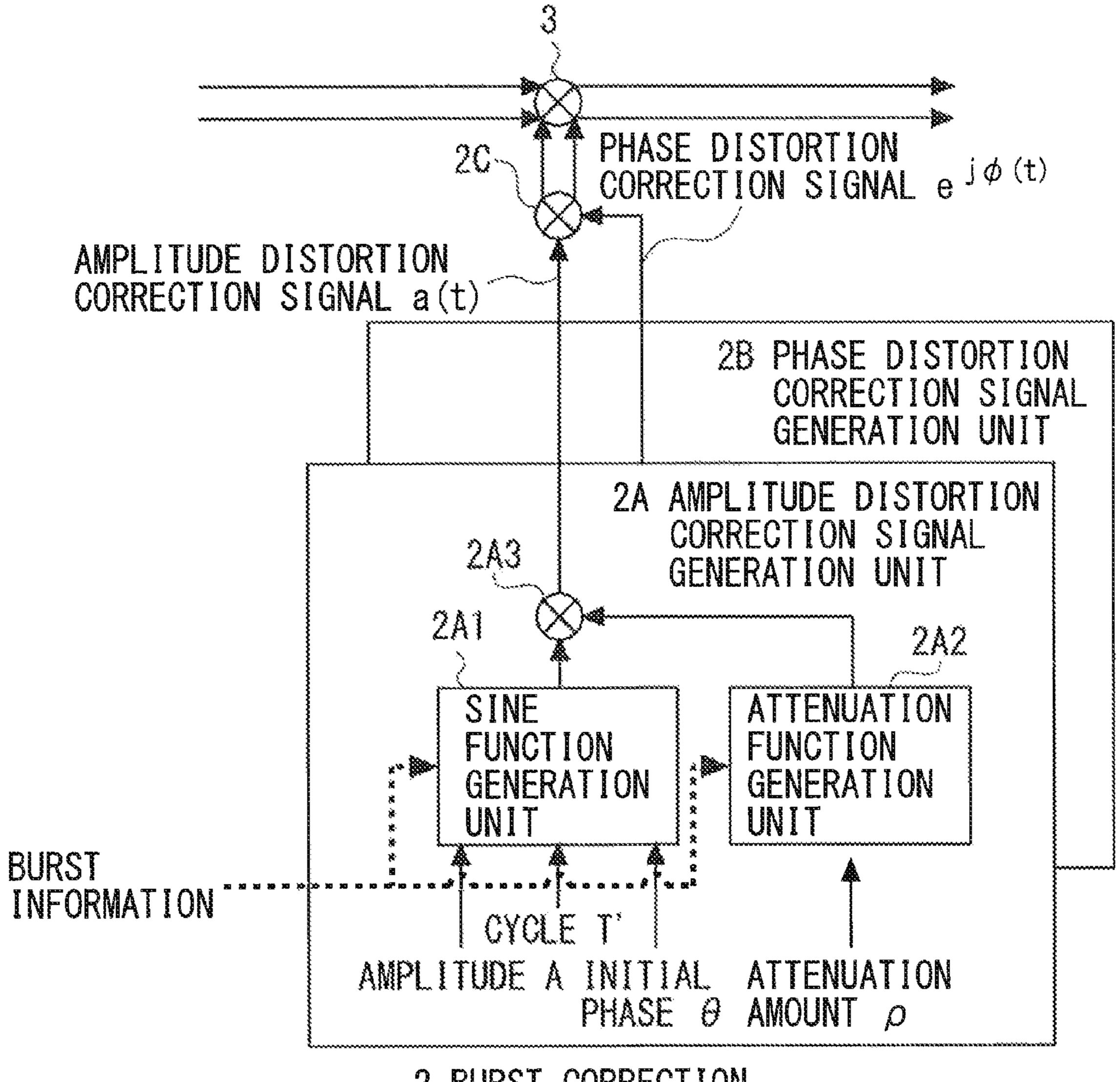
2 BURST CORRECTION COEFFICIENT GENERATION UNIT
