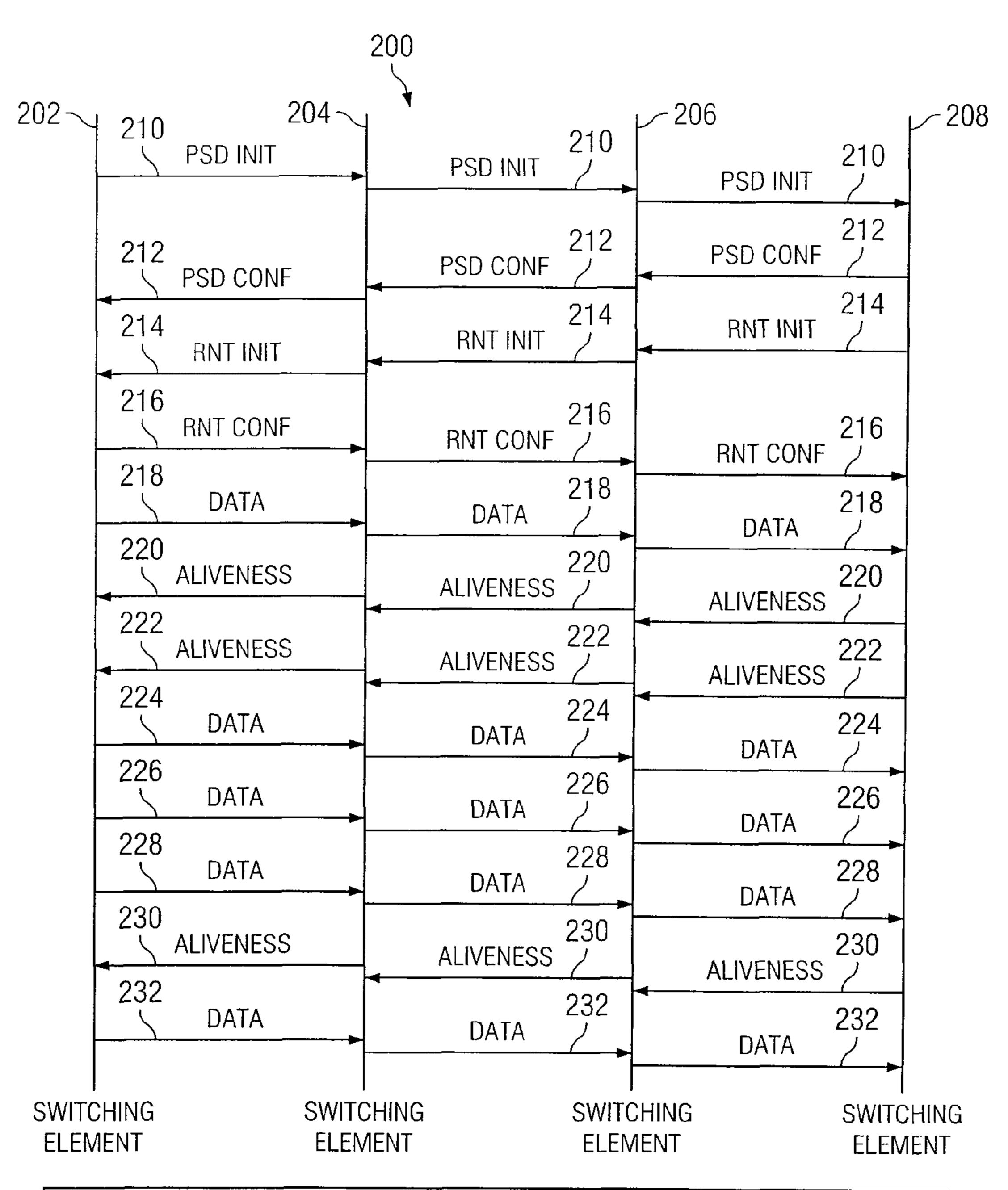
PSD = PROTECTION SWITCH DOMAIN (ESTABLISHMENT OF THE WORKING AND PROTECTION PATH: IDENTIFICATION OF SWITCHING ELEMENTS)
