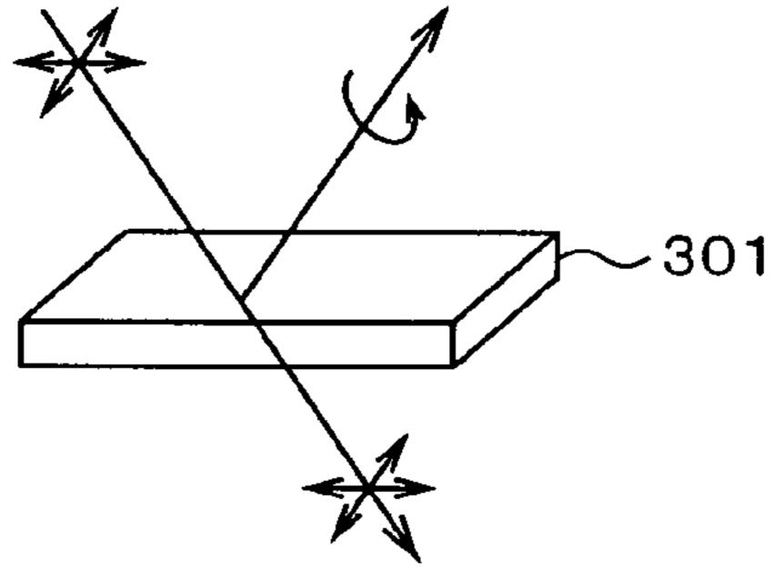
left-handed circularly polarized light, right-handed circularly polarized light having wavelength other than predetermined wavelength, linearly polarized light
