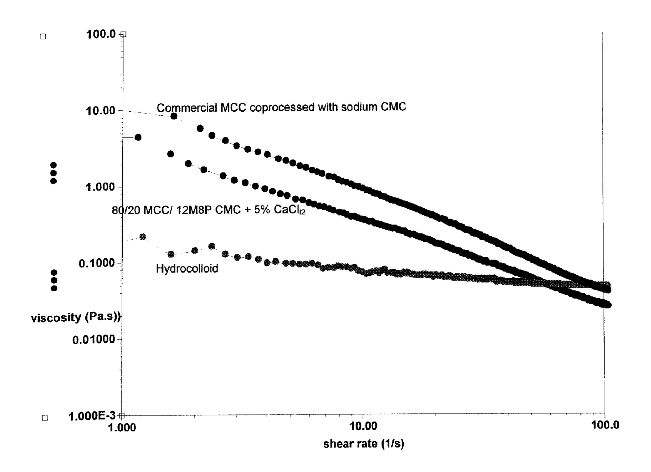
Figure 3: Thixotropy Profile vs shear rate
