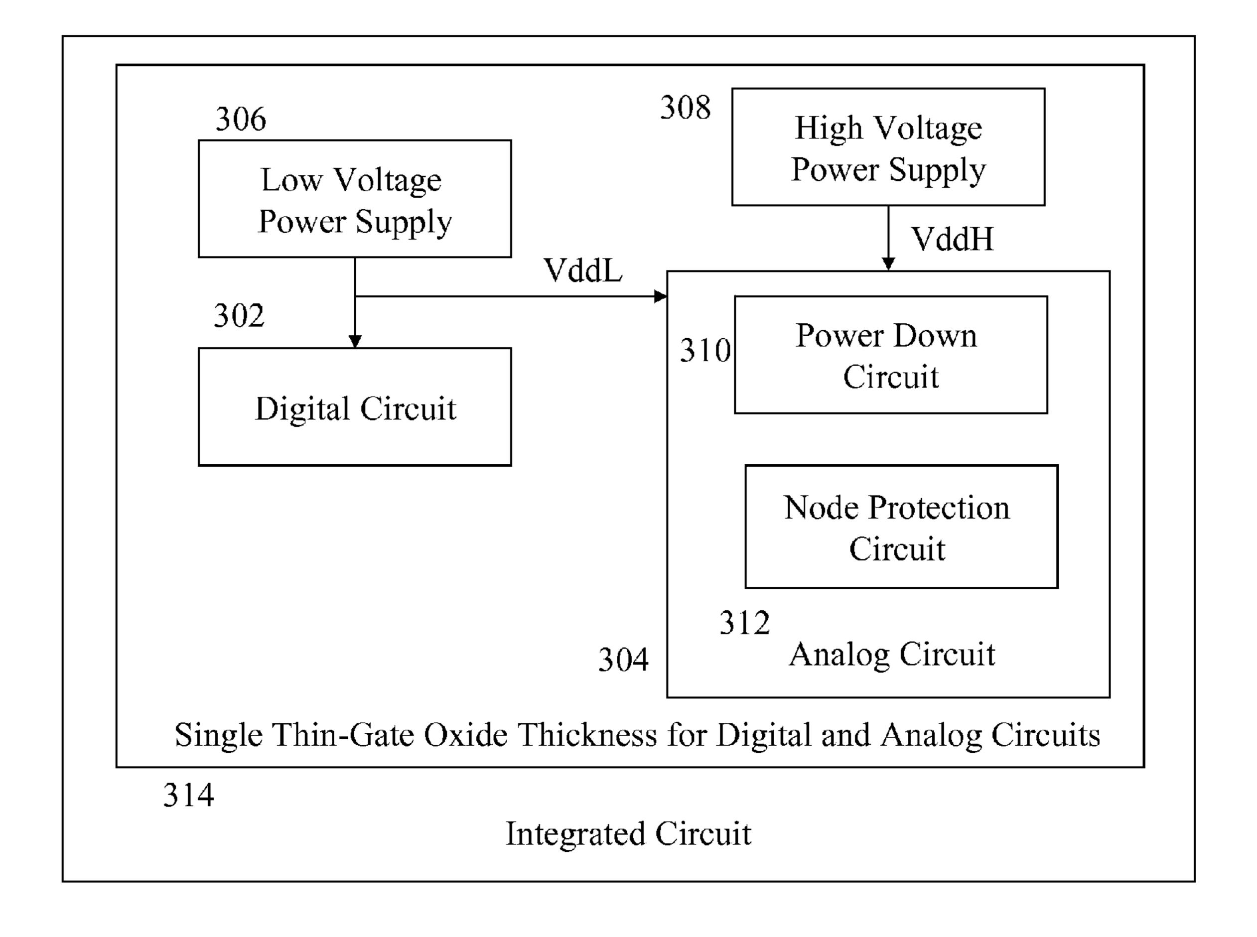
FIG. 6 <u>600</u> Integrated Circuit including an Analog Circuit having A Power Down Circuit with a Dual Power Supply Voltage 201 (VddH and VddL)and a Protection Circuit for Analog Circuit Nodes vddH MP6 MP4 MP2 MP8 MP9 MP3 MP5 MP1 202 vddL vddL A [B]vddL PDN [C]ာ့ on MP12 MP11 MN10 vddLMN8 PDN MP10 MN7 Ibias [O]MN1 MN5 MN2 MN3 MN4 [F]PDN MN11 MN13 MN15 MN12 MN14 VSS
