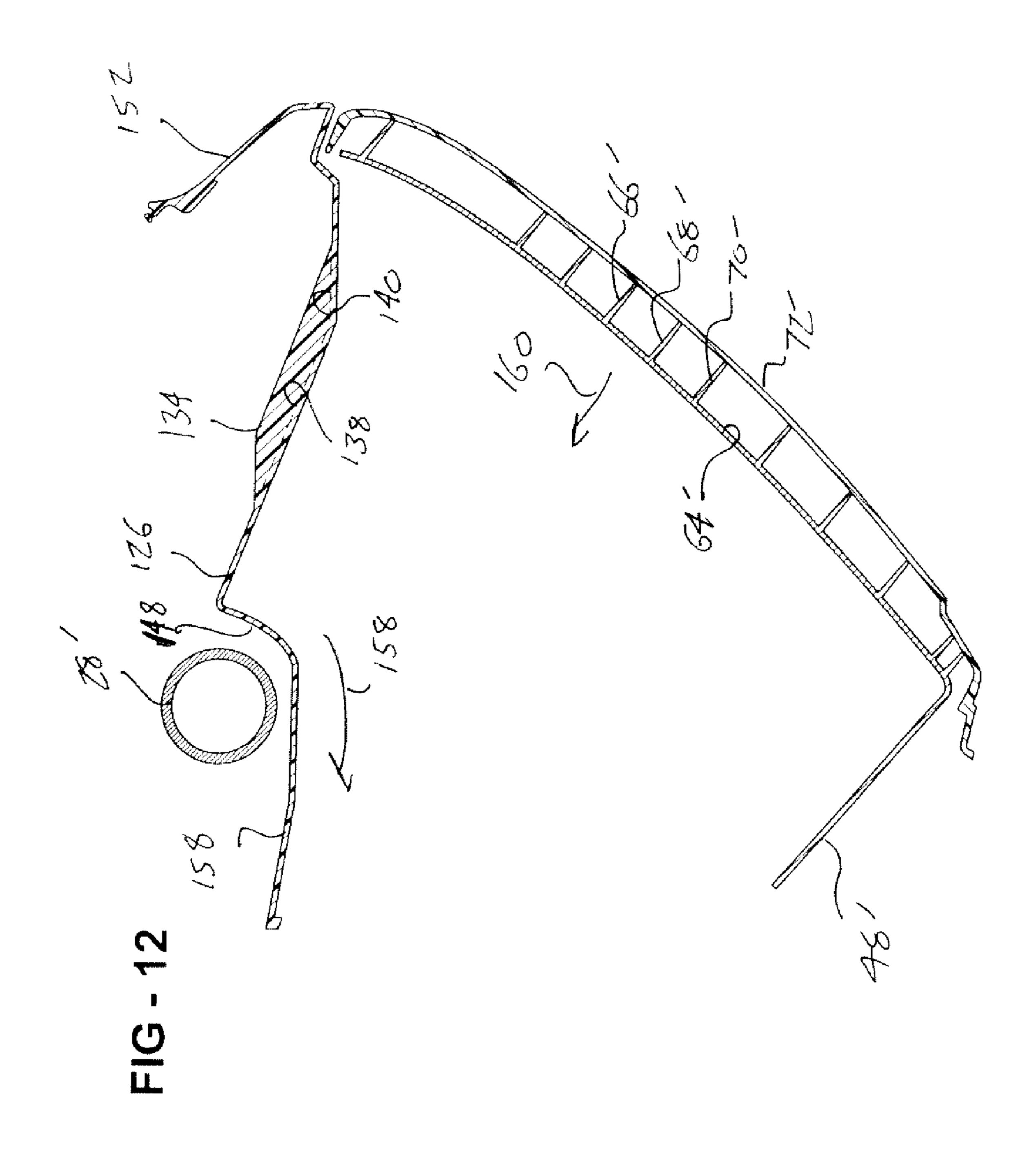
GLOVE BOX ASSEMBLY EXHIBITING KNEE IMPACT FORCE TRANSFERRING STRUCTURE WITH RESPECT TO AN ASSOCIATED VEHICLE DASH/INSTRUMENT PANEL AND REINFORCING BAR AND INCLUDING REMOVABLE STRENGTHENING RIBS FOR TUNING OF CRASH SAFETY CHARACTERISTICS
