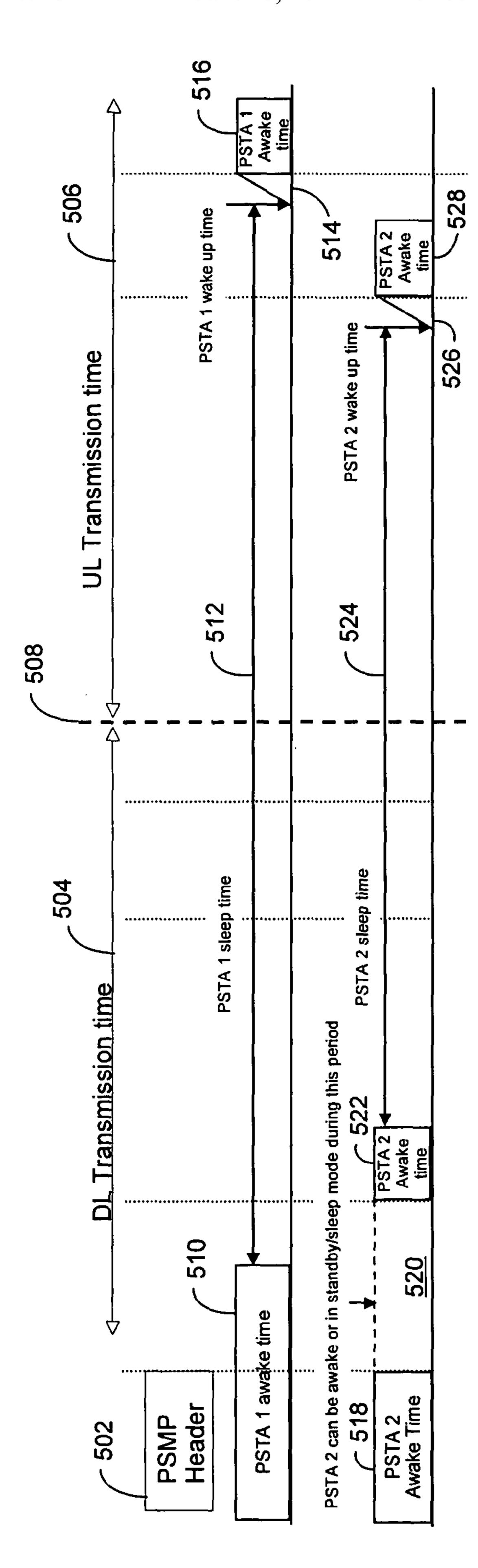
Transmitting a frame identifying uplink and/or downlink transmission periods during a frame sequence for one or more nodes in a wireless network, the uplink transmissions being scheduled after the downlink transmissions within the frame sequence.
