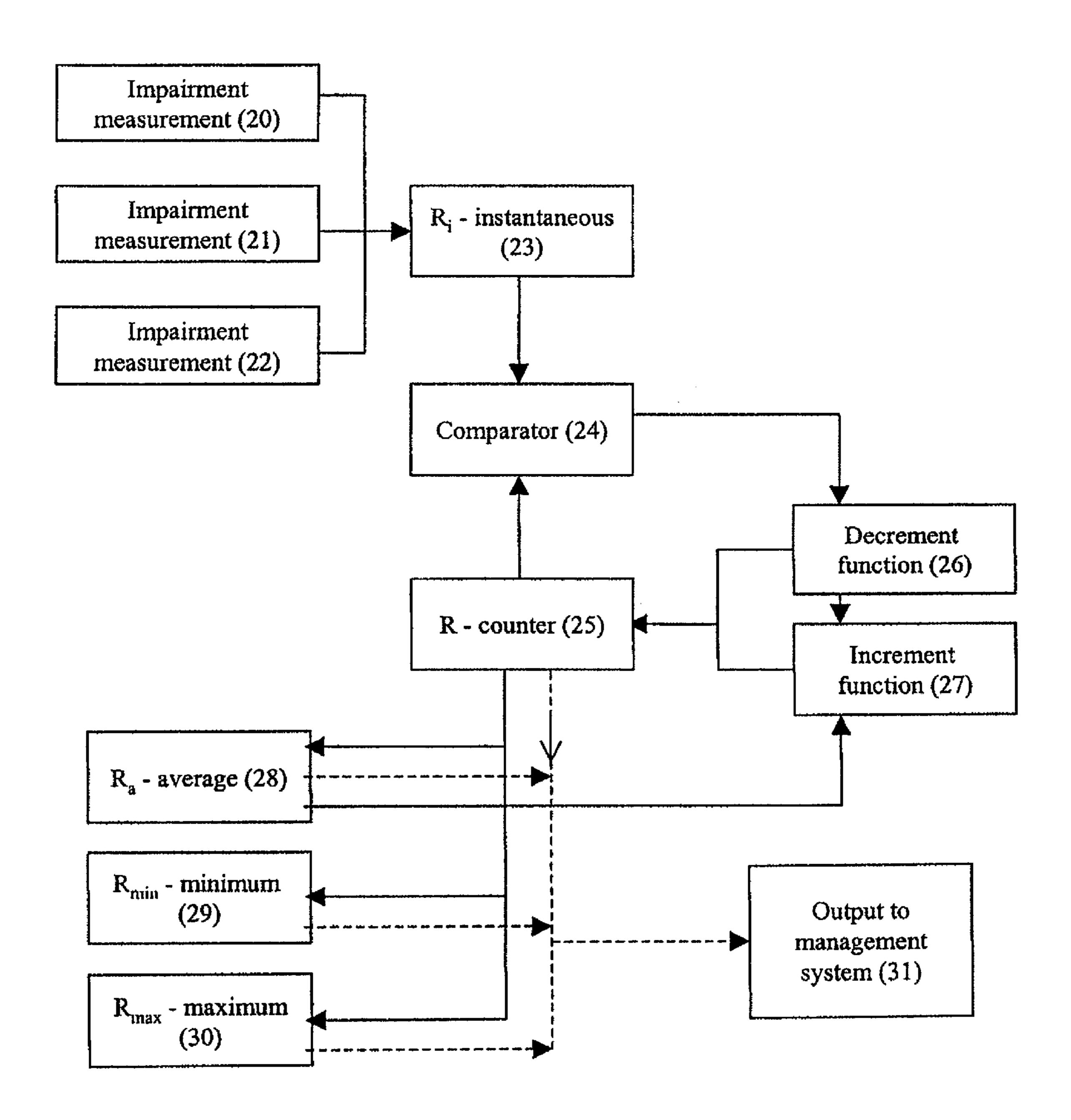
Figure 4 - Architecture of Quality Monitor
