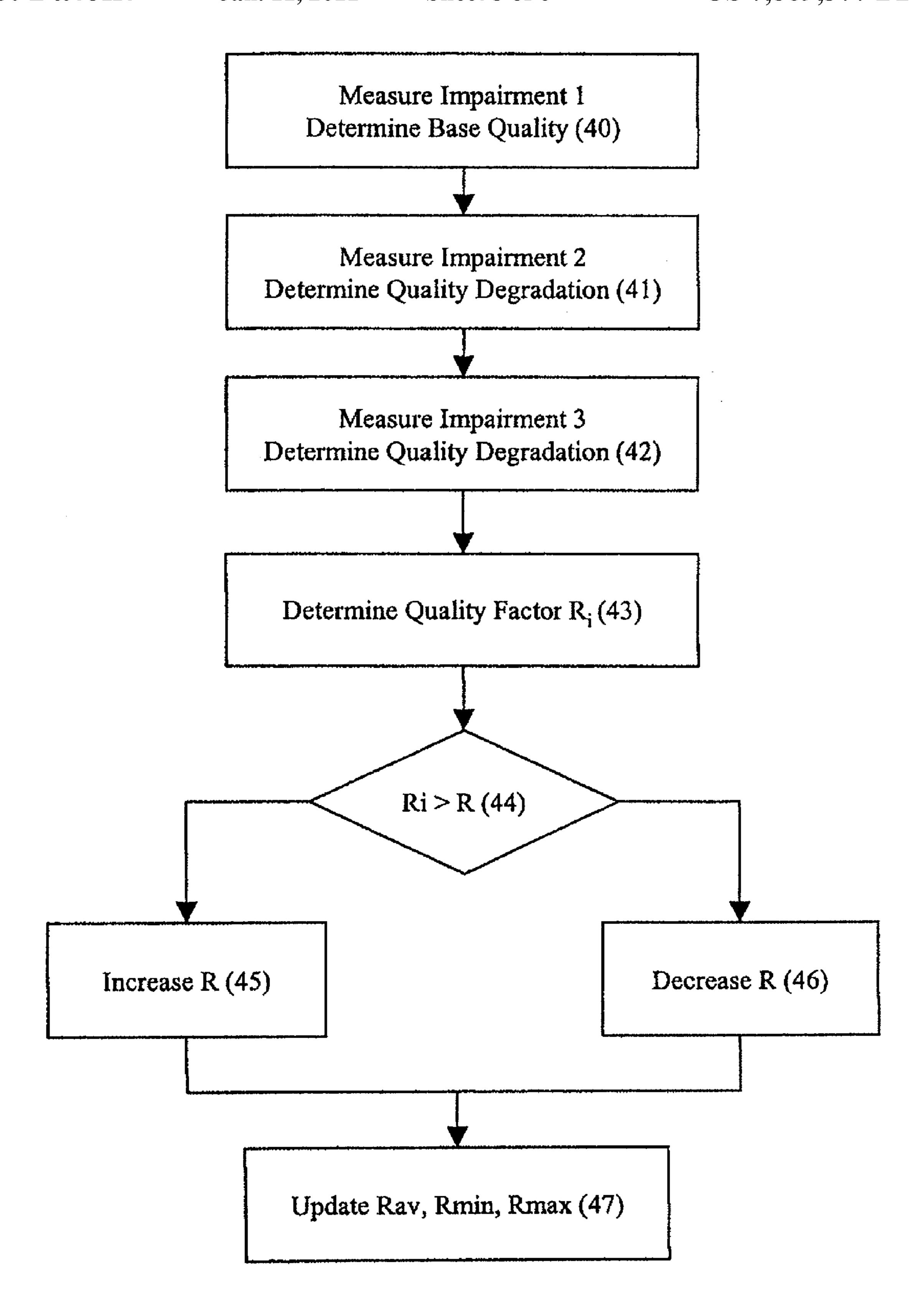
Figure 5 - Flowchart for Quality Estimating System
