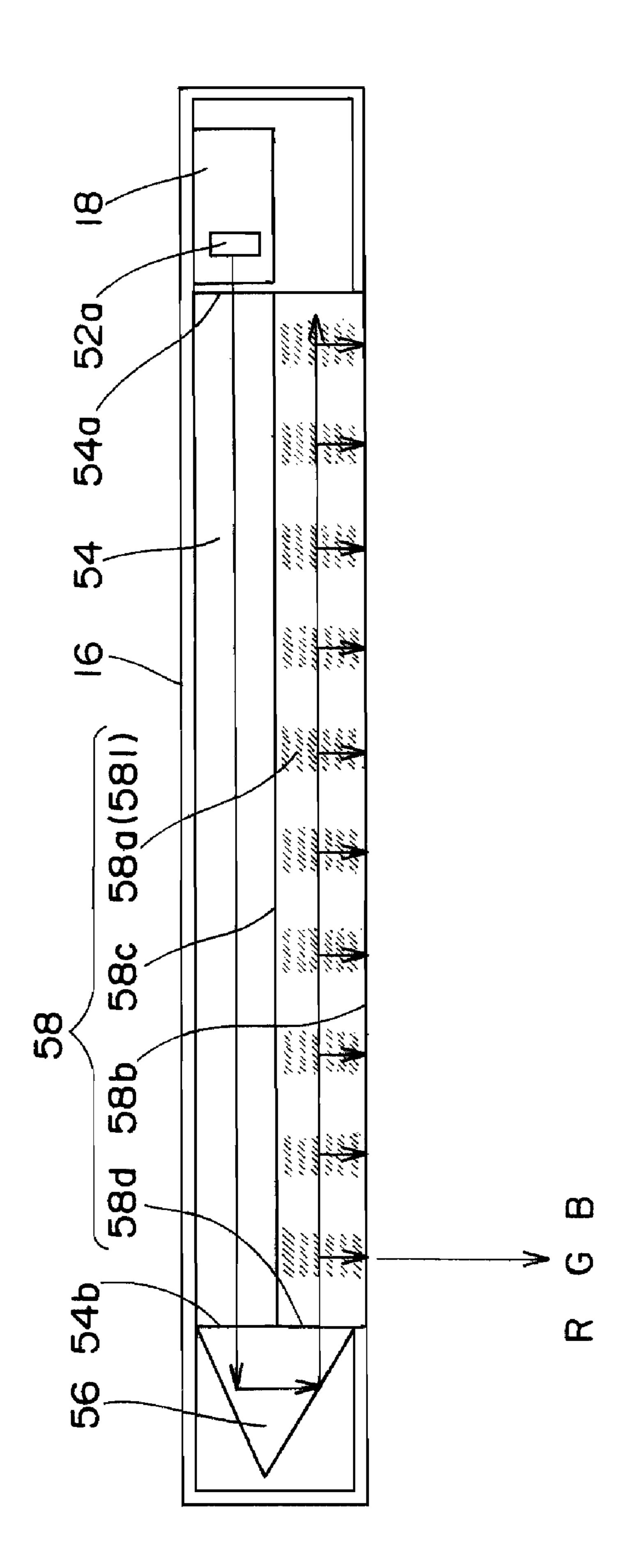
PLANAR LIGHTING AND LCD DEVICE WITH A LASER LIGHT SOURCE EMITTING A LINEARLY-POLARIZED LASER BEAM, OPTICAL MEMBER TO PARALLELIZE THE BEAM AND A PLATE-SHAPED LIGHT GUIDE FOR EMITTING PART OF THE BEAM
