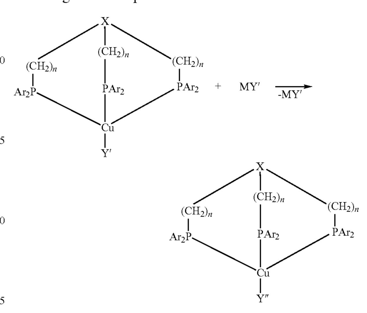
Y' is, for example, chlorine or bromine, Y" is the anion corresponding to the alkoxy, aryloxy, alkylthio, arylthio, alkylamino, dialkylamino, arylamino or diarylamino radical, and M is a monovalent metal, for instance silver(I) or an alkali metal, e.g. sodium or potassium.
