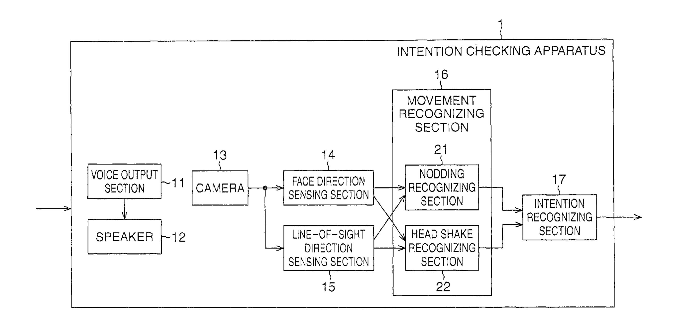
APPARATUS  $\mathbf{\alpha}$ HEAD SHAKE RECOGNIZING SECTION 16 DIRECTION SENSING SECTION 15 LINE-OF-SIGHT
