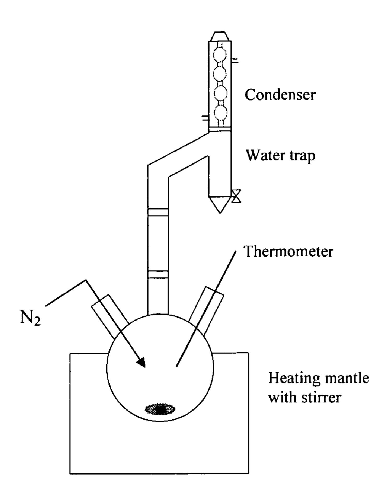
Figure 1. Apparatus for preparation of modified hyperbranched polymers.
