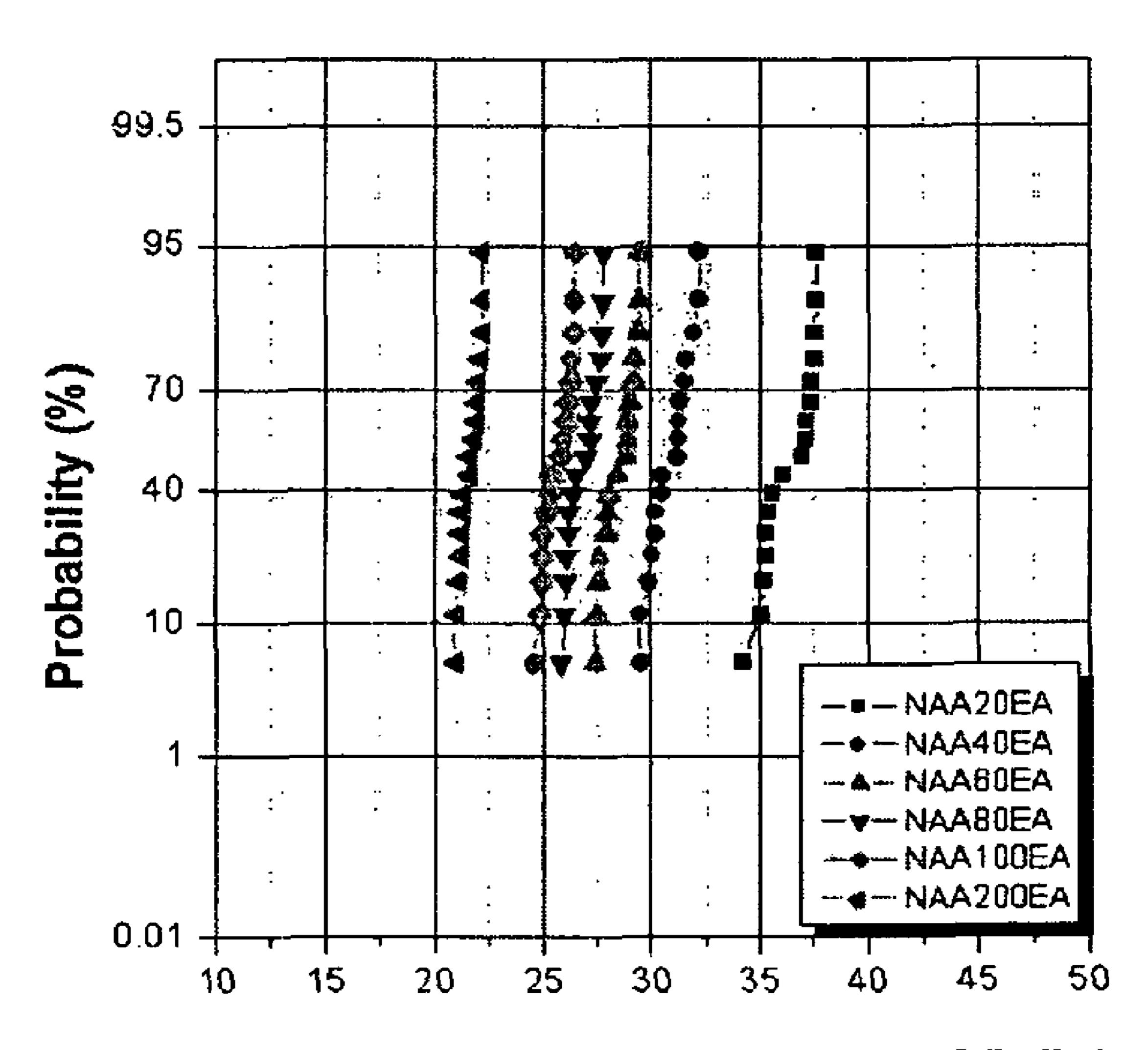
Island Diode Junction Leakage (uA/i-dio)
