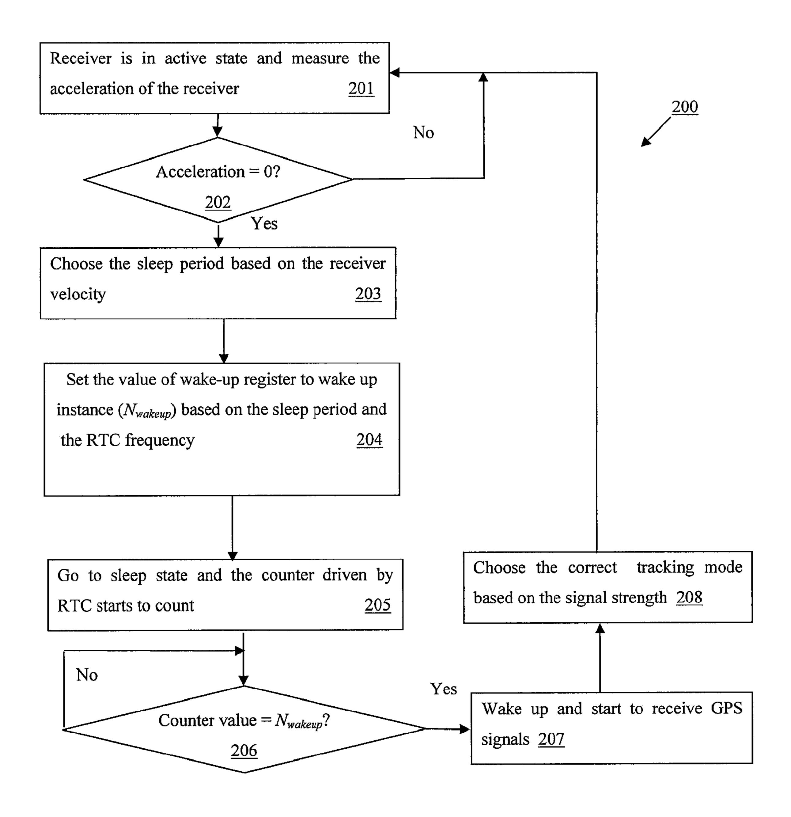
FIG. 2 Flowchart of the low power tracking process
