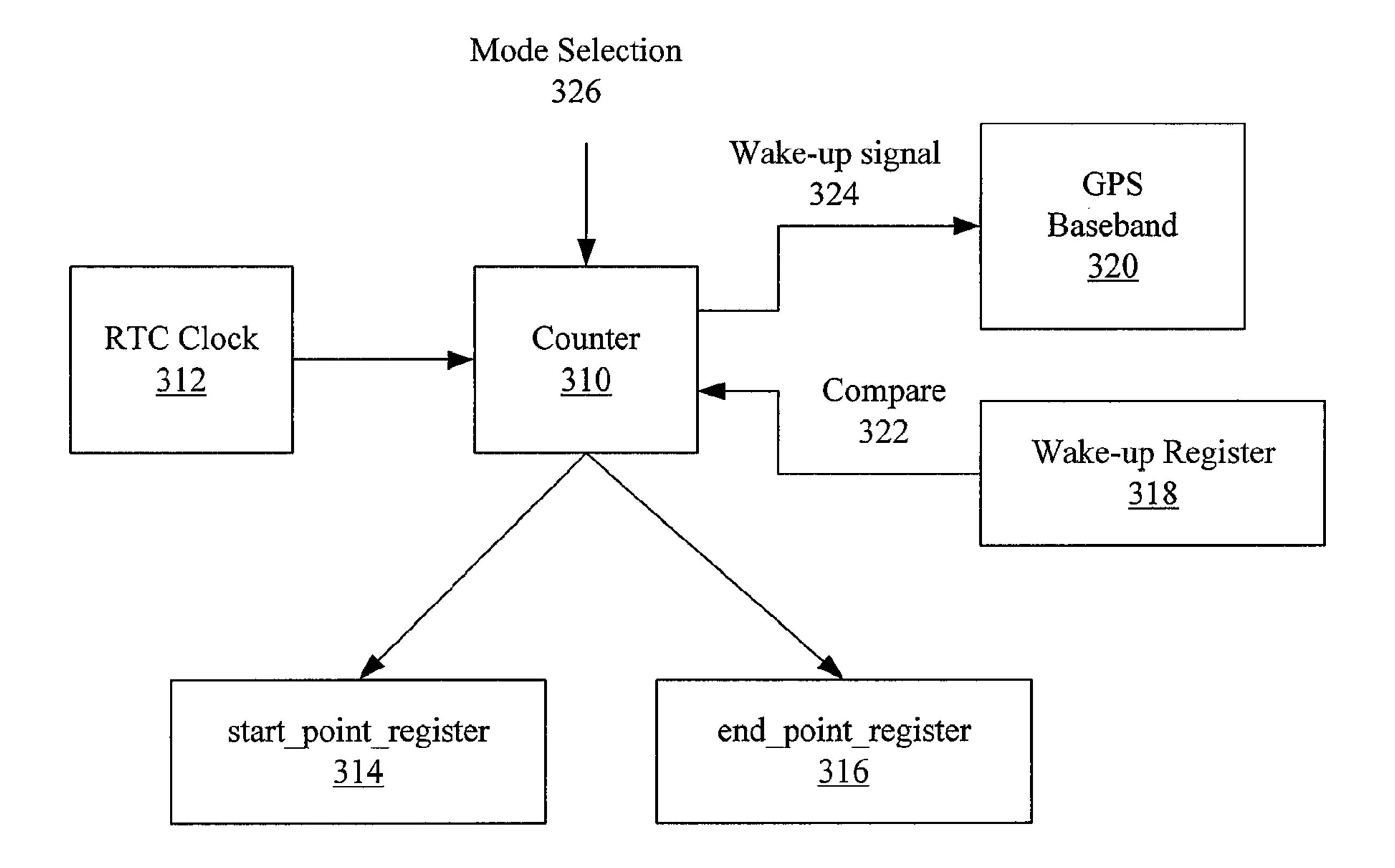
FIG. 3 An embodiment of RTC counter for wake-up control
