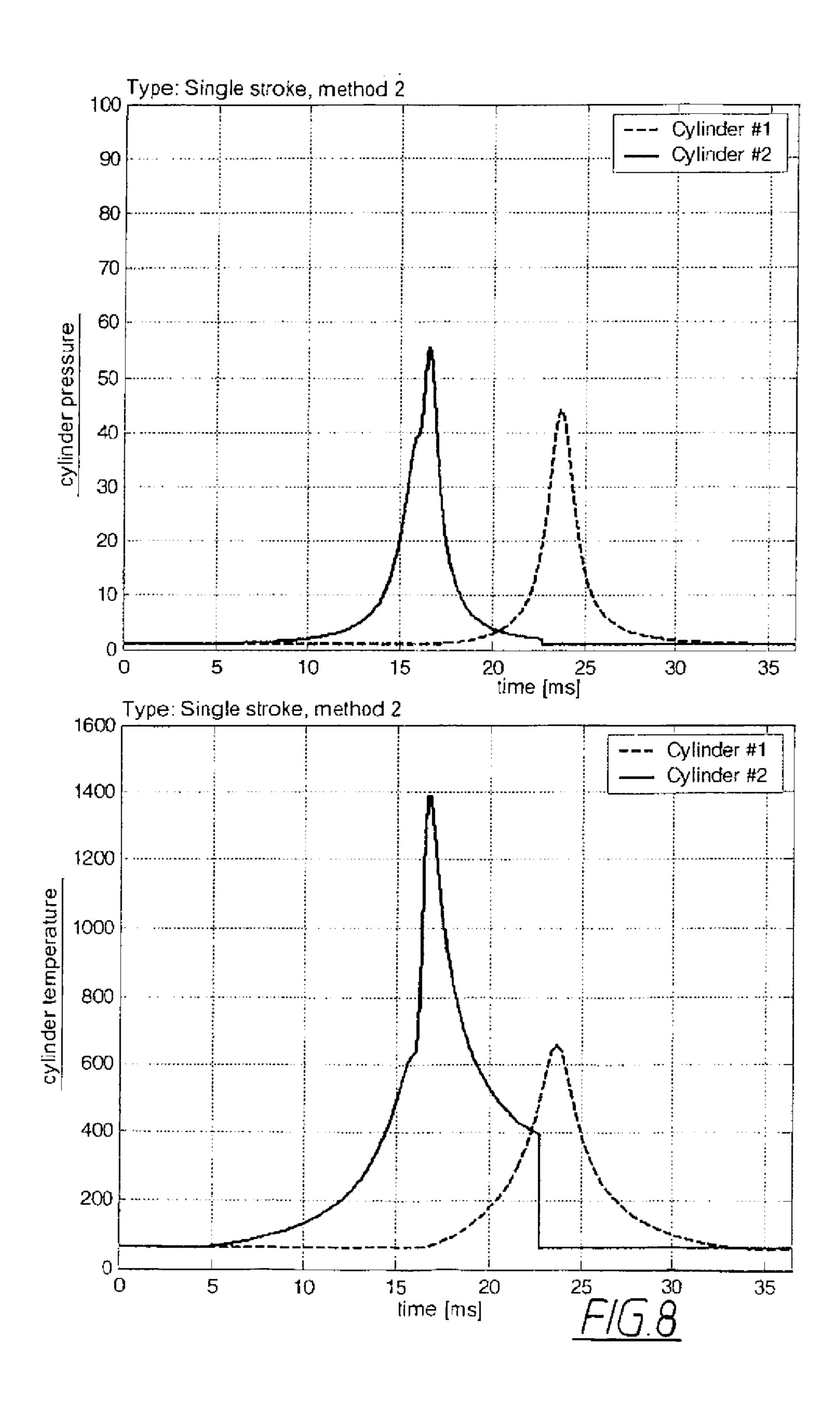
Type: Single stroke, method 2. Cold start -30°C
