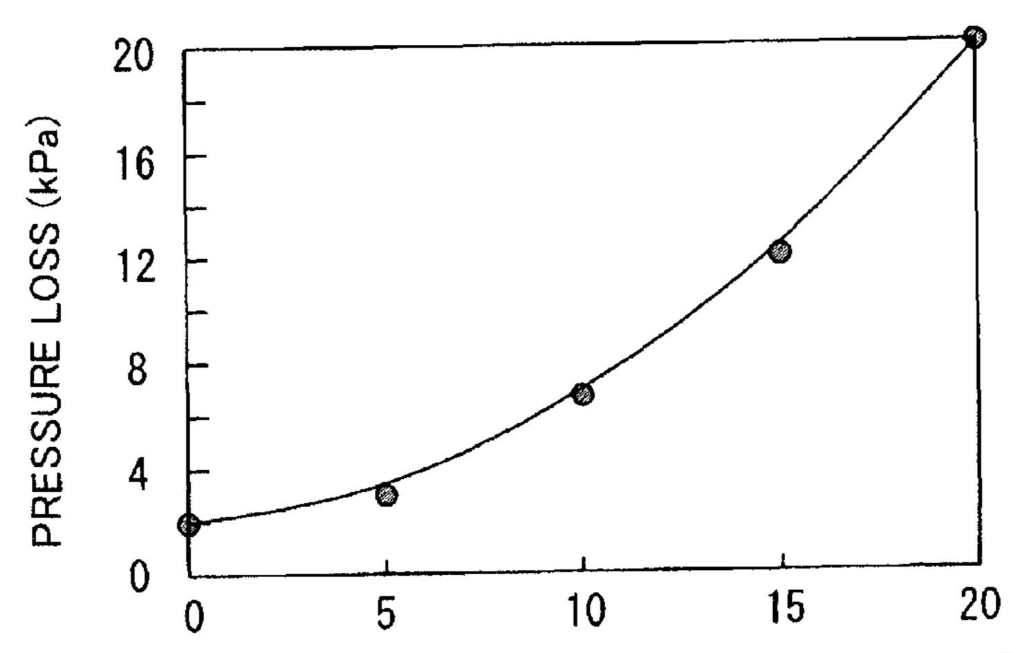
PERCENTAGE OF PORES HAVING PORE DIAMETER OF LESS THAN 2  $\mu$  m RELATIVE TO ENTIRE PORES (vol%)
