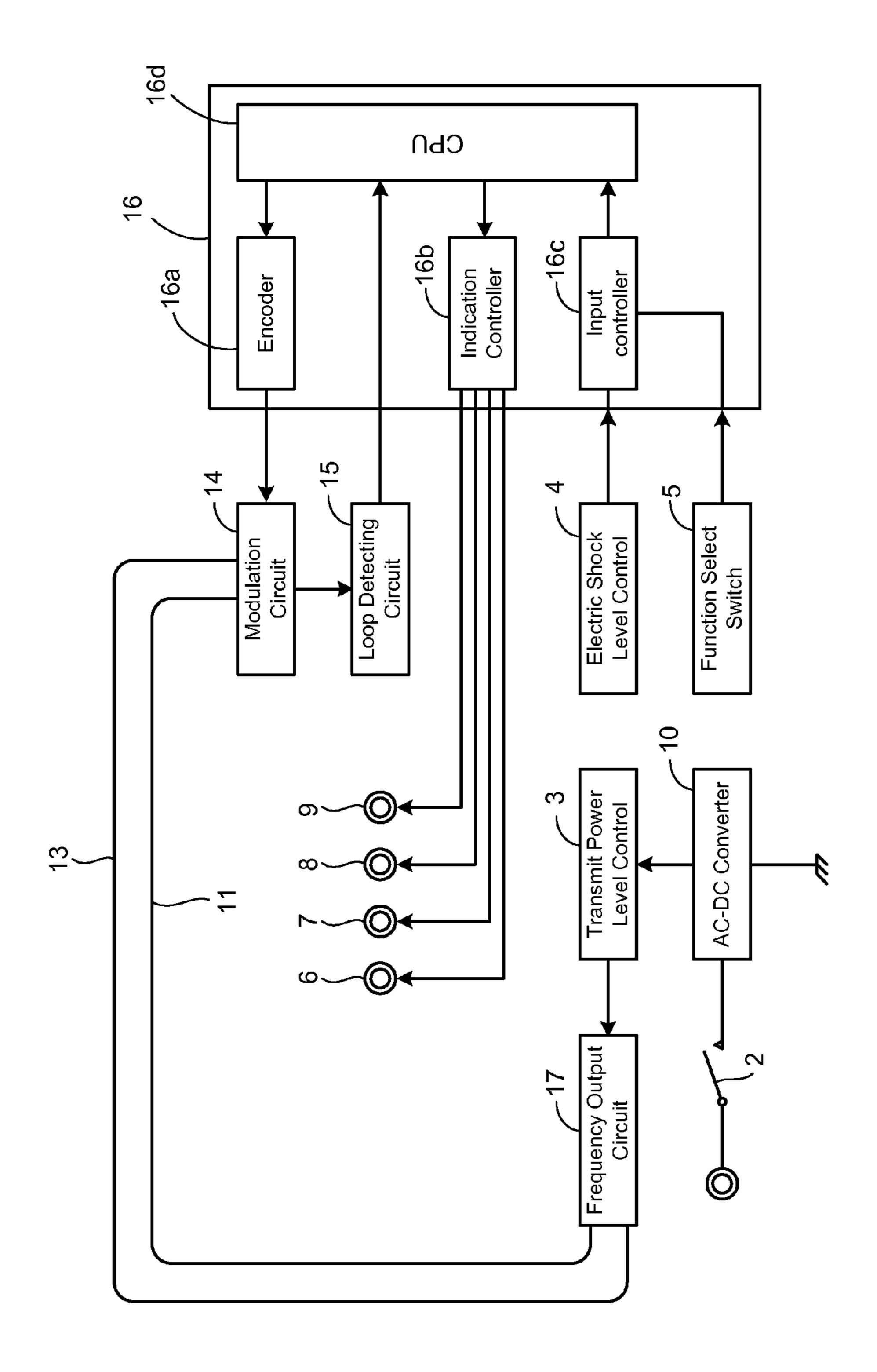
Transmitter block diagram
