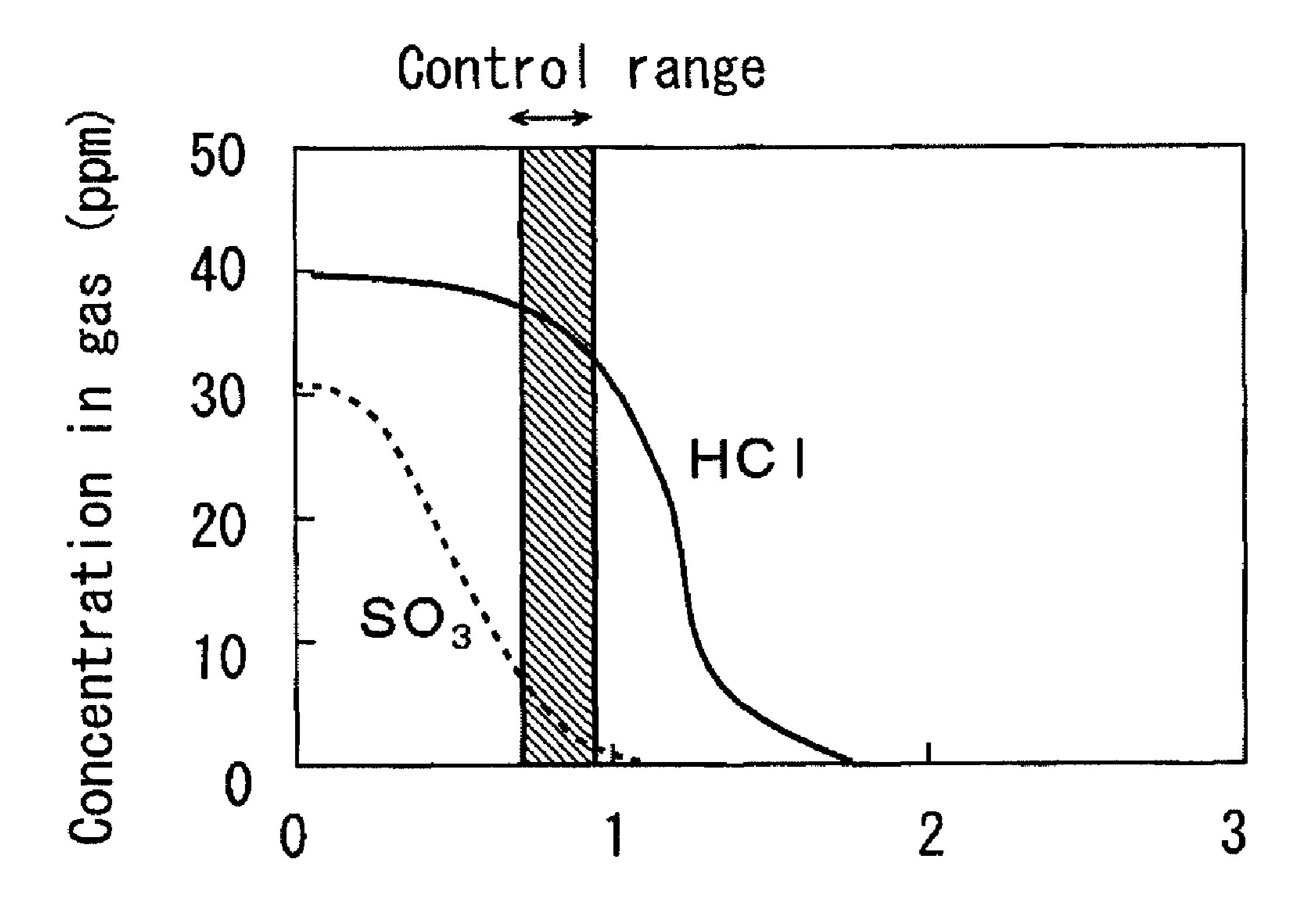
Neutralizing agent supply amount in mole equivalents with respect to SO3
