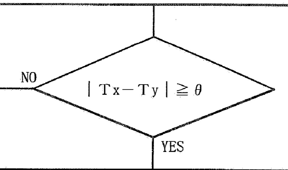
Adjust measured temperature Tx of upper pyrometer to estimated substrate temperature Ty.
